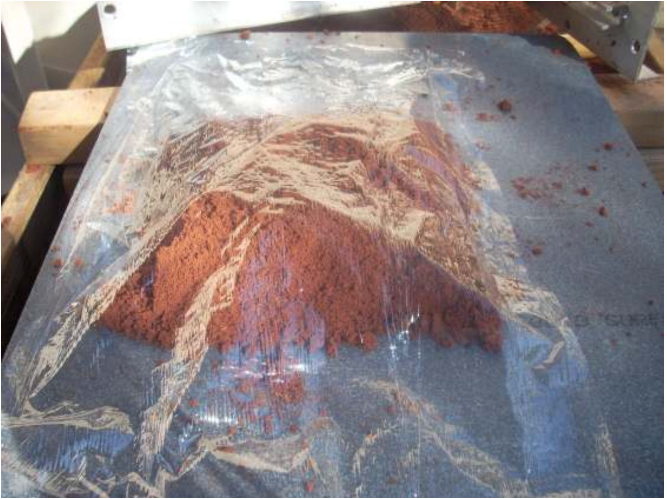
The drag is lifted up and a sheet of plastic wrap is placed over the sand.
