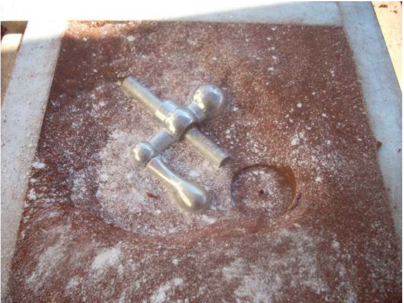
This time it all worked. You can see the sprue pin's imprint in the drag. I have not cut in the gate yet.
