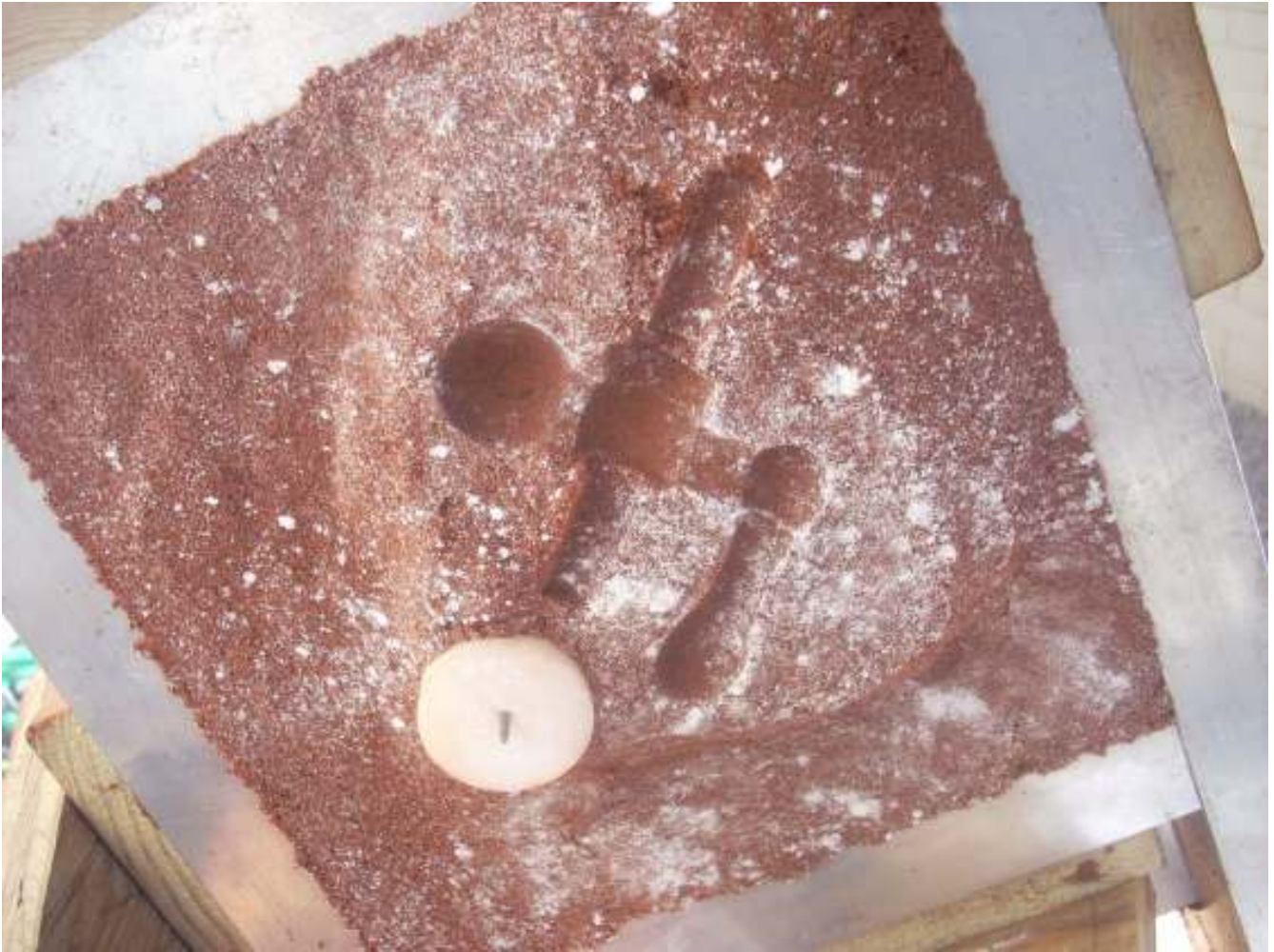
The cope imprint came out nice and clean. All that was left was to pull the sprue pin and cut my funnel.
