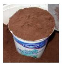
1. Fill a tapered-side cup with sand being careful not to tamp it down.
