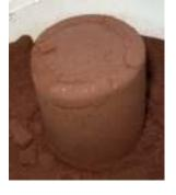
4. Turn the cup over close to a flat surface and let the contents plop out. If the shape holds, the sand is good. If you end up with a crumbled pile of sand, it is not strong enough for casting.
