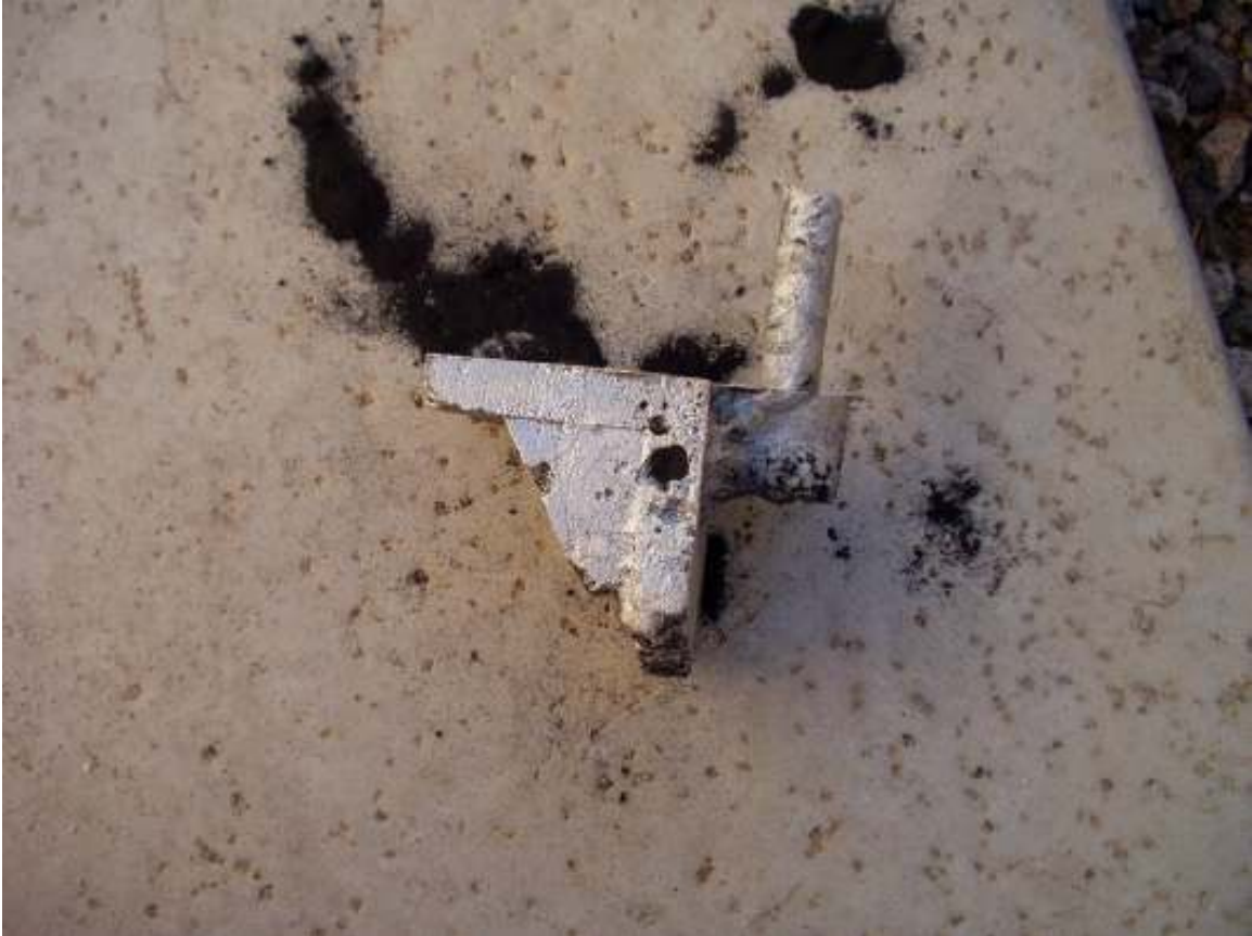
The gate and sprue are part of the pattern.
