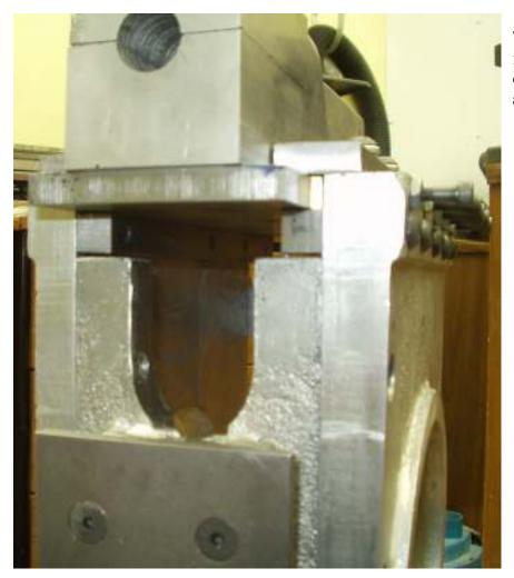
The right side has the gib which is brass. Adjusting the gib is easy because of the 5 adjustment screws.
