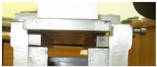
Sorry about the camera not being level, but you can clearly see the slide ways, brass gib on the right, and top clamps. The shims and UHMW tape are barely visible.
