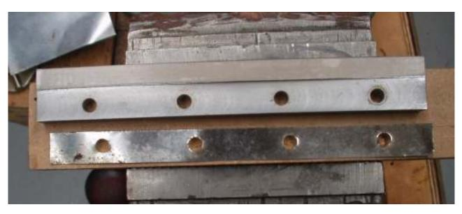
I cut one 0.016", two 0.006", two 0.004", and in the end had to cut a 0.0015" for the right side. The left side was fine without it.
