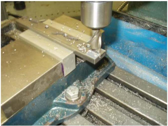
I set my mill vise and took a clean up cut on the soft jaws. My left clamp was then clamped in place. I am about to cut a step 0.025" deep and 0.600" wide. Note the white patch on the right end of the bar. It is a scrap of UHMW tape.
