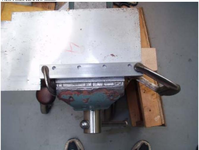
I was lucky to have cut that step in the clamp bars. It enabled me to clamp a piece of MDF in my bench vise, fit the first clamp bar against a piece of 0.004" shim stock, and clamp down. I then ran my "F" letter drill down each hole, through the shim, and into the MDF. The holes therefore are perfectly aligned and undistorted. Without moving the C-clamps, I used an Exacto knife to cut the shim. After each shim was cut, its orientation was marked.
