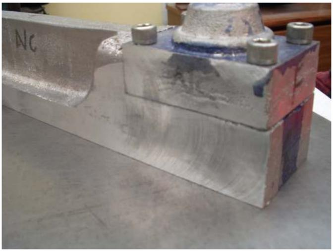
Drilling and tapping the 4 holes was nothing special. I then remachined the sides so the cap would be the same width as the ram. Here you see the side with a little shrink blemish in the ram cap.
