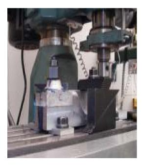
The cap has been fitted to the ram and clamped down. Note that I am again using machined pads to insure that the ram casting is parallel to the X axis and to the table top. I have placed a 20 thou aluminum shim between the cap and ram body. After I drill and bore out the pivot hole, this spacer will be replaced with smaller shims to provide a sliding fit on the pivot bar.
