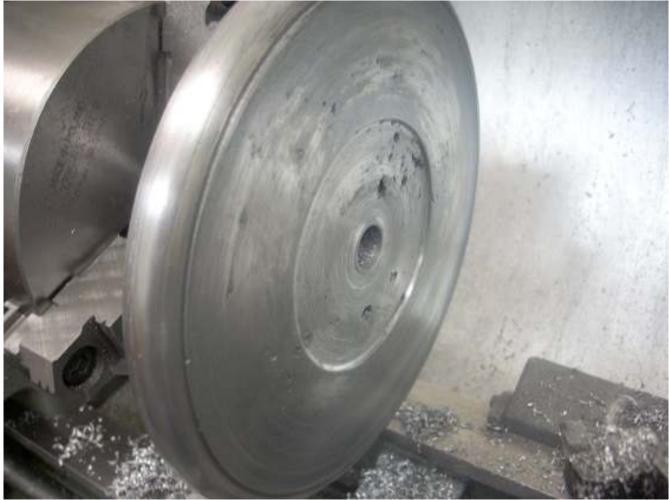
I trued up the outer face. The recess came from machining out an area with a fair amount of shrinkage. I didn't want to remove more metal to have it completely flat. Who knows, maybe I'll glue in a curved arrow in this recess to remind me which direction to turn the handwheel.
