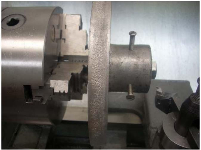
This time I'm using a mandrel secured by screws but will only face the end of the hub and turn the perimeter of part of the hub true. I would have cut more of the hub but my <sup>1</sup>/<sub>4</sub>-20 grub screws have not arrived from Enco yet. Those bolts sticking out are not "cutter friendly". In fact, they aren't knuckle friendly either.
