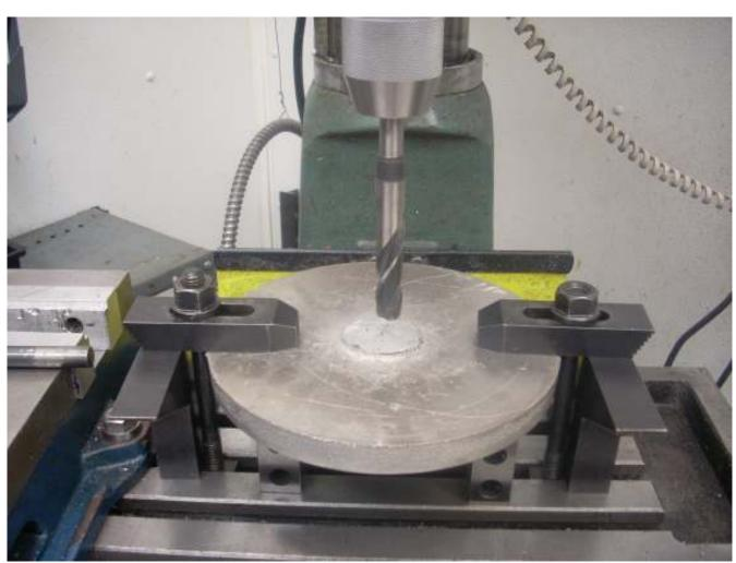
Last time I went for a bored hole that was a nice sliding fit on the mandrel. Not such a good idea since the mandrel distorted slightly and jammed in the hole. This time I'm simply step drilling with a  $\frac{1}{4}$ ",  $\frac{1}{2}$ ", and finally a 5/8" drill. Quick and a bit more room in the hole.
