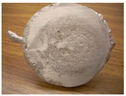
The casting came out usable. The center of the bottom was a little higher than around the end. This is probably because the melt dropped down the sprue and struck the sand at the bottom of the mold. That pushed down the sand resulting in a bulge in the casting.
