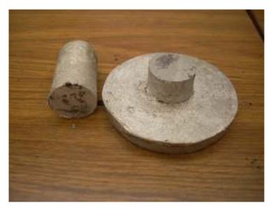
The sprue was sawed off at about 3/4". That leaves plenty of room for a finished length of 1/2".
