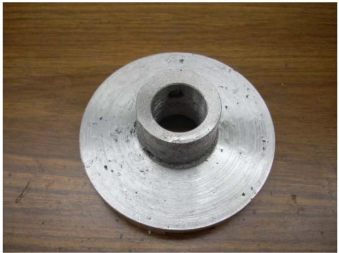
Here you see the finished feed crank. Note that the bore is not centered in the hub. It may not look great but works OK. What is important is that the bore is perpendicular to the bottom face. You can see some surface imperfections which are not pretty but the part is usable. These are not gas bubbles.
