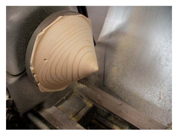
It made a mess of my lathe and shop, but I turned a very nice looking cone. The hole in the side of the cone is from pilot holes for wood screws that hold the wood to the faceplate.
