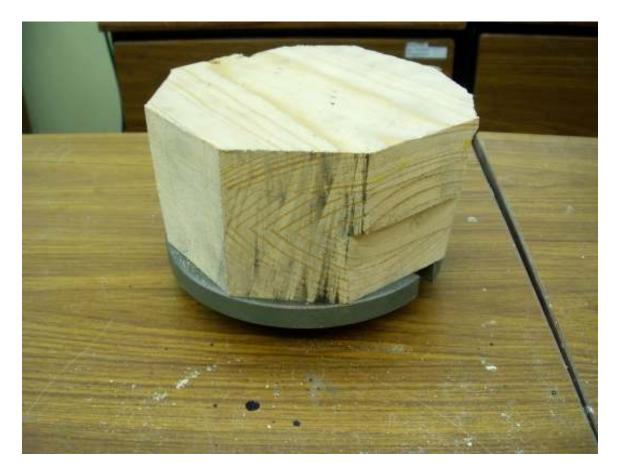
I started with a stack of glued up pine and mounted it on a faceplate.
