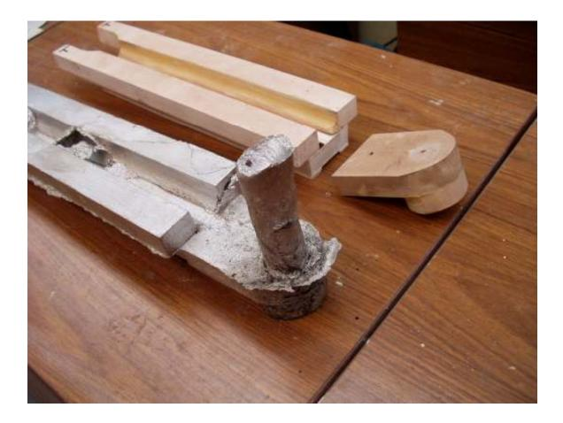
Here you see the sprue and gate next to their pattern. They seemed to work well. My goal was to have a nice even flow into the casting. The downward force of the aluminum falling down the sprue was absorbed by the void below the sprue. The extra wide gate slows the flow while distributing it across the casting impression.
