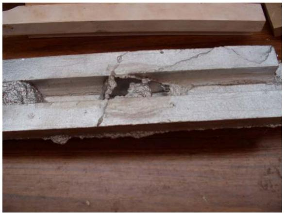
Here you see the fault line in the cope. Lots of sand fell down to provide more room for aluminum. If this was the extent of the damage, I could have milled it out.
