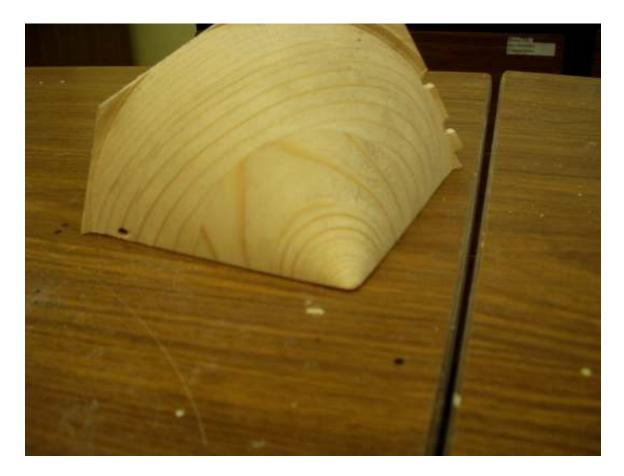
I then used a handsaw to cut the cone in half. This was followed by cutting out the sectors shown in the drawing. In the end my gluing job was poor and bit of wood fell off. That was easy to fix but the resulting sectors just did not look so good. Not much learned on this one but glad I did not use these side lobes.
