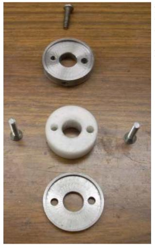
Nothing special about the lathe work. The top and bottom are CRS. The recesses are 0.05" deep and cut with a boring bar. The plastic is Delron®. The plastic scale is 0.005" thick so there
