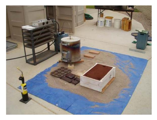
The flask is ready for pouring. I have about 75 pounds of sand in that flask. It was not easy to carry from my sandbox seen in the background to the casting area. It was murder gently lowering it down to the ground. My back is a bit tender now. *Next time* I will ram flasks this size on my wagon and then wheel them over. I will still have to flip the drag over but that is not nearly as bad.
