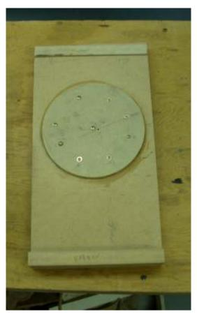
Here is the pattern before I cut the hole. One lesson learned is to write lots of "dummy" instructions on the pieces to be glued together. The draft is only 1 to 5 degrees and it is easy to stick a piece of wood on upside down. It also prevents me from using a finished strip of wood as a glue spreader stick.
