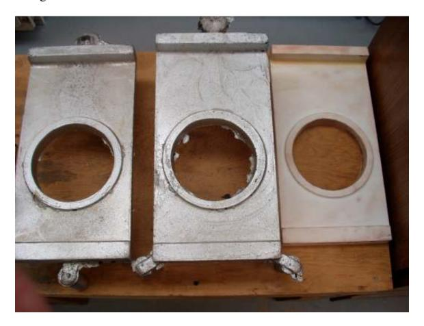
These are the faces that everyone will see. The center casting has some damage near the hole. It is ugly but will not effect the part's strength. A bit of Bondo and paint can cover this sin. At this time, I'm not interested in casting another side plate.
