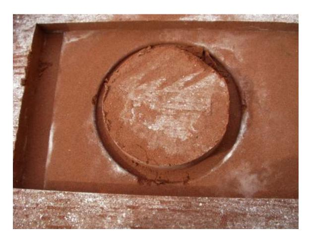
With the pattern drawn, you can see some damage to the edge around the hole. I did not ram hard enough. On my second casting with this pattern I rammed much harder. I used my narrowest tool and worked the sand into the pattern at a 45-degree angle. It greatly reduced this problem.
