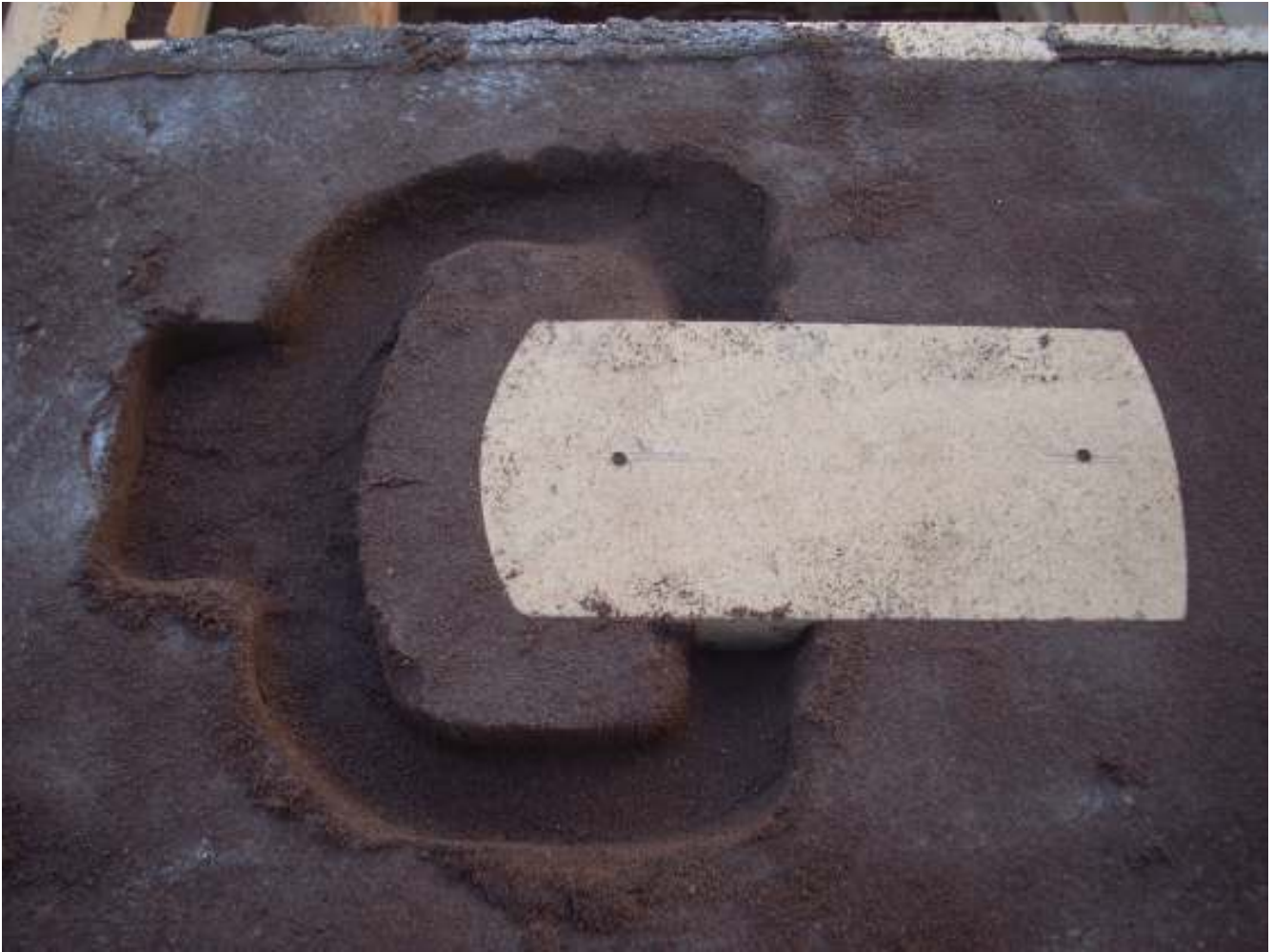
I chose to pull the gate system first and do my cuts with the clapper box pattern still in place.
