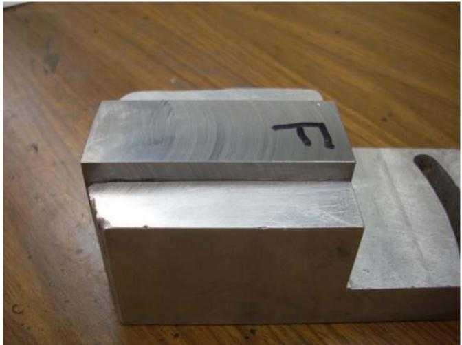
When the clapper is in the bottom of the box, I can't see any light between the two and it sure does feel snug. The clapper is not perfectly square because if I put it in the box upside down, it does not fit. We are talking about an out of square condition of less than 0.000 5".
