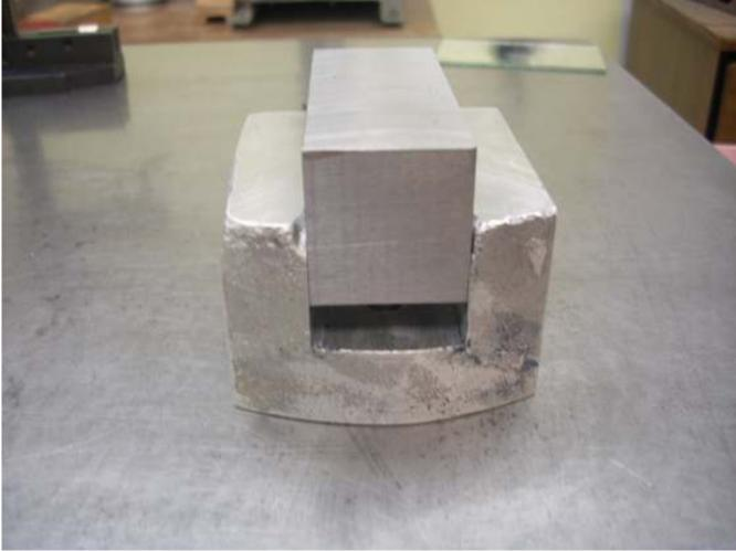
It doesn't take much taper in the box to prevent the clapper from dropping all the way down. If I had cut the clapper to match the top width of the box, it would have been much higher in the slot. Oh well. My machines and my skills certainly have their limitations. At least I can get a great fit for the bottom half of the box.
