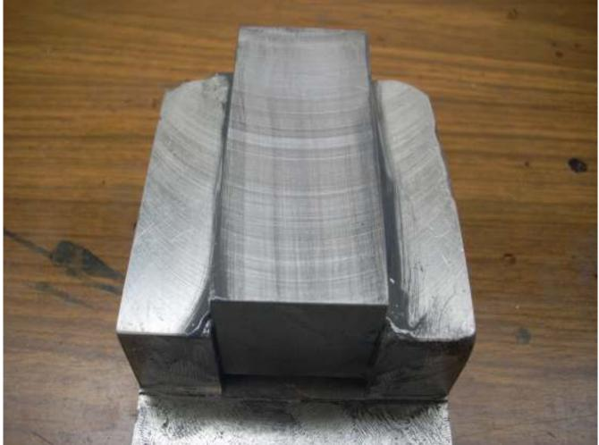
It took some time moving the clapper back and forth, but it slowly removed aluminum and the block sank into the box.
