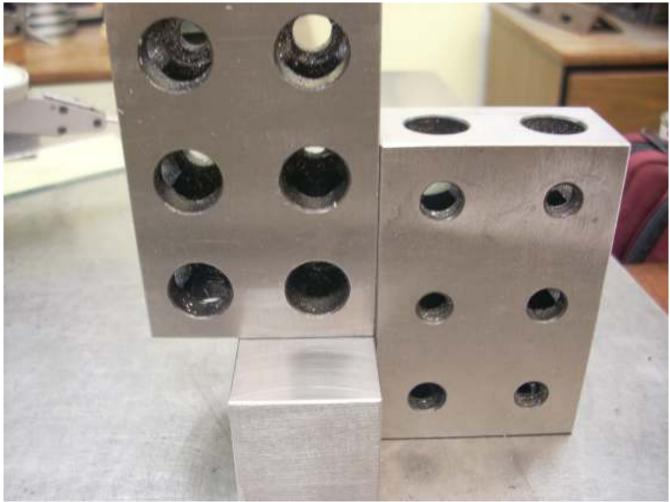
To test for squareness, I used two precision 1-2-3 blocks and looked for light between the 3 blocks. All was nice and tight so my block is reasonably square between the top face and the right face. The block was rotated 180° and the diagonally opposite corner was tested. It looked just as good.
