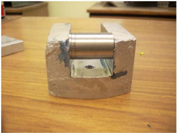
I used my spacer blocks to monitor my progress as I removed small amounts of aluminum from both sides of the box.
