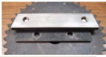
I want the distance between the bars to be 5/8" as measured against the sprocket. This is accomplished by just placing a 5/8" parallel down and pressing it against the first bar.
