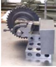
Next the sprocket was laid out. This was done by fitting it to a piece of scrap 3/4" round stock. The round stock was then clamped to a V-block.
