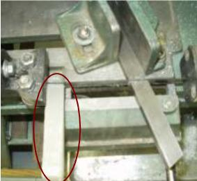
One thing of note here is the block of paraffin wax on the left side of the picture circled in red. My bandsaw blade teeth first cut across this wax and then cut the CRS. In this way cutting lubricant is freshly carried into the cut. The cut end of the bar had an even coat of wax on it indicating that there was plenty of wax present.
