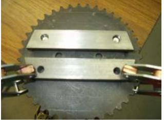
The the second bar is pushed against the parallel and clamped in place. You can see the holes of the parallel in the gap.
