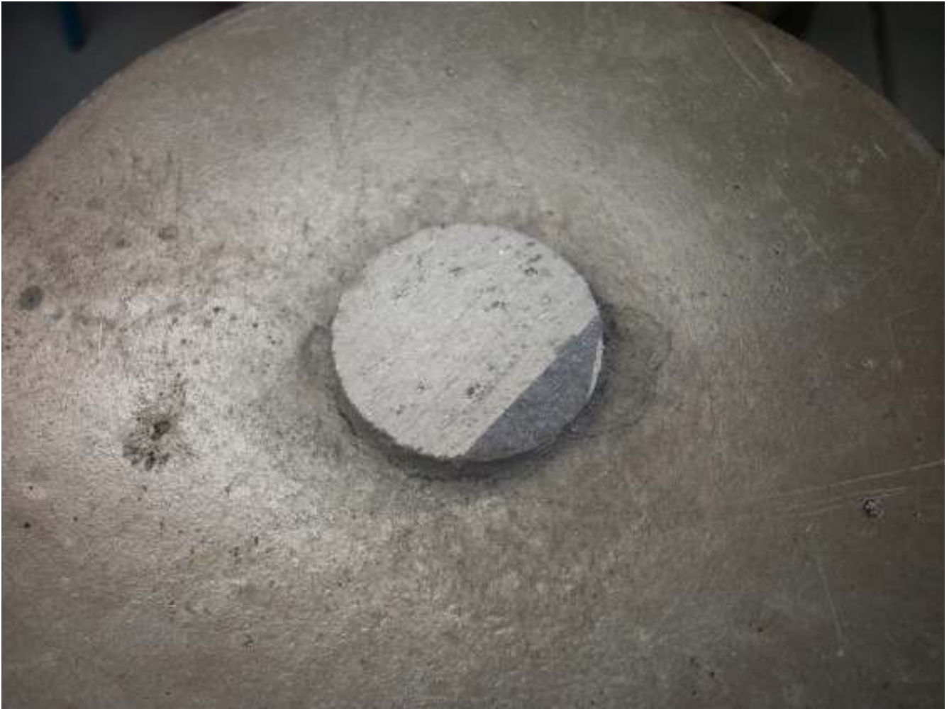
With the sprue cut off, you can better see the shrinkage.
