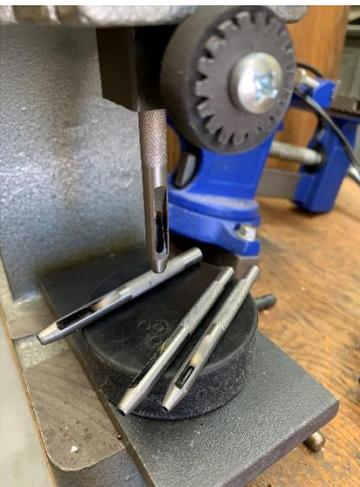
The next attachment inspired by Unisawyer was a set of punches. I had these hand punches and found that they fit into the bore. I'm using a hockey puck to support the stock as I punch through. If this is too soft a surface, I have some expanded PVC, a piece of hardwood, and some brass. One of them should work.
