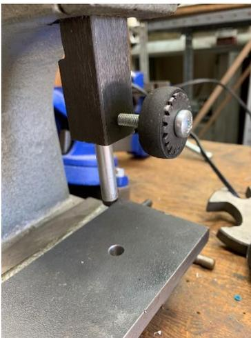
Just to try out his last suggestion, I fitted a 3/8" rod to the ram. Then I aligned the plate's 3/8" hole.
