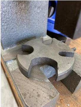
The one attachment that came with the press was this disk. I never needed the cutouts and when I used a patch of the solid area, the disk would rock. It didn't give me a lot of confidence.
