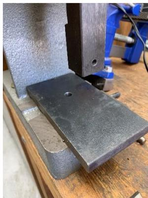
Ultrasimple attachment #1 was to put that disk aside and put down a plate of hot rolled steel. It has a 3/8" hole in it. Future attachments can have a 3/8" rod on the back to engage this hole. No more rocking.
