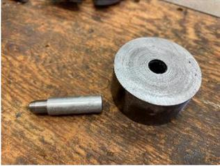
Unisawyer made up pair of “presser plates” (timestamp 9:23) with the back turned down to 3/8”. I had a puck of CRS in my junk drawer. I drilled and reamed it 3/8” and then pushed a pin into the hole. It won’t be as strong as a turned down spigot but will be fine as long as I don’t push too hard on the unsupported part of the face.
