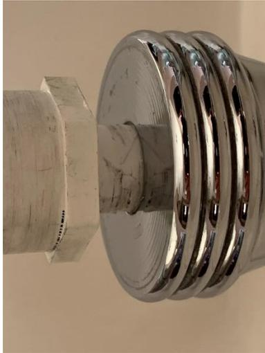
Using my lathe for alignment, I held the coupler in my 3 jaw chuck while the spigot fit over my tailstock's drill chuck. It was then easy to hand turn the 3 jaw chuck while holding onto the spigot. As the spigot's internal threads cut into the plastic, I fed the tailstock in to maintain alignment.
