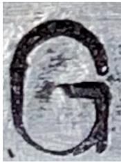
The “G” was hit a little high. Note the line thickness at the top of the letter versus the bottom.
