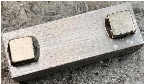
One magnet is near the top and the other is near the bottom. They gently pull on the stamp and prevent rotation due to small vibrations caused by handling. I can smoothly rotate the stamp and it will stay put.
