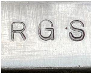
By turning the stamp slightly counterclockwise by eye, I made the “S” almost vertical. This time all three imprints are bottom heavy. Oh well...
