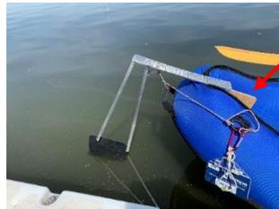
A wooden plate wedges between the gunnels to secure the frame.
