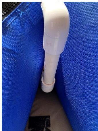
Because there is so little surface exposed to the flow of water when the kayak is moving forward, there is little force trying to rotate the frame upward.
