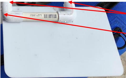
8. Place the assembly on the plate, flat side down. The top of each coupler is aligned with the top edge of the plate. The left side of the left coupler is aligned with the left edge of the plate. Use the pencil to trace around each coupler on to the plate.
