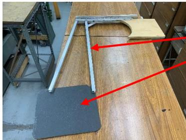
My previous prototype has an aluminum frame with a plastic plate for the skeg.
