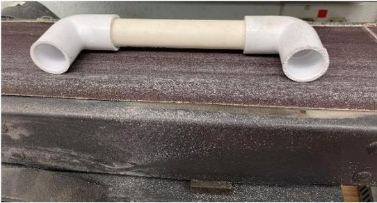
7. If you have a belt sander, gently place the assembly down on the moving belt and abrade off flats on the flanks of the couplers. The goal is to have two "L" shaped flats about 1/4 inch wide.
