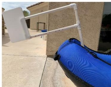
In shallow water, rotate the frame up.
