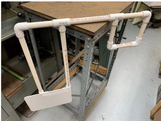
11. Complete the assembly process being careful to keep all pipes and couplers on the same plane.
