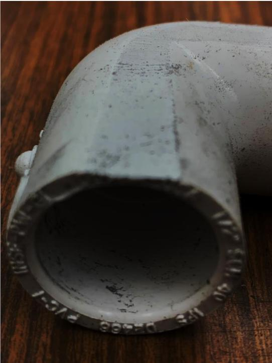
This machining can be performed with a hand file. Just keep a close eye on the flats to be sure they are of uniform width. A straight edge will verify they are on the same plane.
