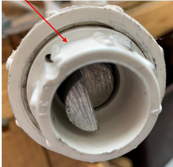
Then I drilled into the face with my tap drill going through my previously drilled hole.
