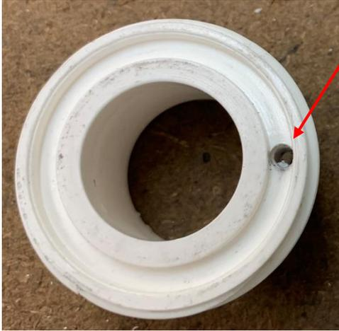
I took a spare PVC union and drilled a tap hole in the desired location.
