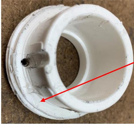
Then I held the part in my lathe's 3-jaw chuck and removed the flutes, plus squared up this face.
