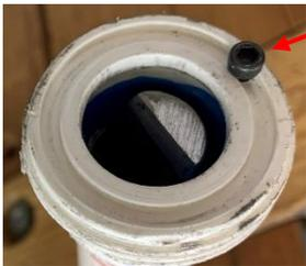
The solution was to add a pin to one side of each union and drill a matching hole on the other side. I drilled and tapped the first hole 6-32 and installed a Socket Head Cap Screw. The other hole was drilled large enough to easily accept the screw's head.
