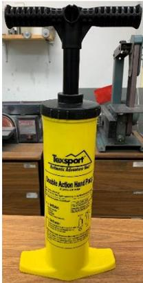
This is my Texsport low pressure/high volume air pumps. It is useful when pumping up my inflatable kayak. When I bought my second-hand kayak, it came with this second-hand pump. I did not get any airflow until the plunger was about 3 inches from the bottom. Lots of wasted motion and not a lot of air.
