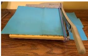
Using my trusty paper cutter<sup>2</sup>, I cleaning cut on the mark. The goal was to have the plastic sheet fit snug top to bottom. This ensures that the piston can't get under or over the sheet where it will catch.
