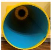
Then, I rolled up the sheet and again slid it down the bore. This reduced the inside diameter by about 0.01 inches from top to bottom. There is a small vertical overlap but it is harmless.
