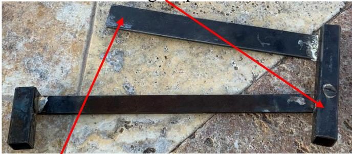
The other “finger” pivots on the cross arm. I placed it into the other square hole, clamped it to the cross arm, and drill a hole through both pieces using an “F” drill. Then I ran a 1/4-20 bolt through and secured it with a locking nut.
