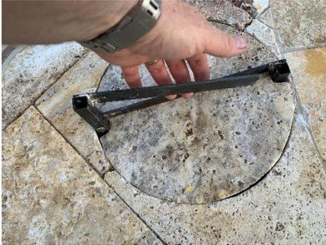
To release the lifter, I lower the cover down on the deck. Then the handle is lowered which pivots that one finger and the tool is free.
