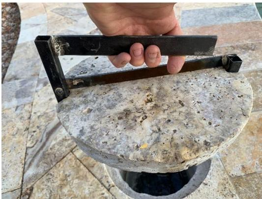
As I lift up on the handle, the pivoting finger rotates in and pulls both fingers to the tapered angles. This locks the cover to the lifter tool.
