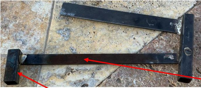
This tool does the trick. The parts are brazed together but they could have been welded. Initially I used Pop Rivets but they were far too weak.
