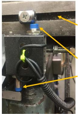
I mounted the X and Y home sensors on the front right corner of the apron.
