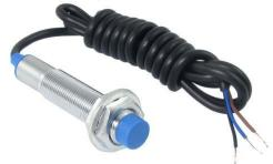
This is a magnetic proximity switch<sup>2</sup>. When iron or steel gets close to the end of the blue cap, it responds by pulling its output wire near ground. Remove the metal and the output becomes an open circuit.
