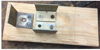
I threw together this dead simple nest from a chunk of 2 by 6 and three brackets. It is heavy enough that the grinder stays put. The sides are spaced apart so that it is easy to just drop the grinder in yet not move too much.
