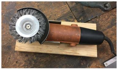
After you turn off your angle grinder, what do you do next? It is still spinning fast enough that it can walk around a work bench. The thought of it falling off the bench and onto my leg is motivation enough for me to hang on and wait until it stops spinning. Not any more!
