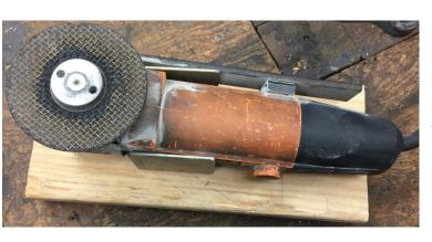
My other angle grinder has a bar attached to the side. It too just drops in place.
