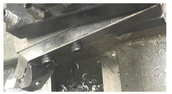
After reassembly of the holder and bar, I ran my screws through. Since it was drilled in place, of course the parts all fit.
