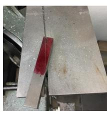
A few words about cutting the CRS bar. I first used Dykem on the surface. With a protractor, I marked a line at 12°. The exact angle is not that critical so  $\pm 2^{\circ}$ is fine. This cut is only to give clearance. I did not want a sharp point on it so the end of the resulting taper is about 1/8 inch thick.
