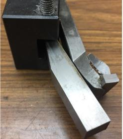
I first set the cutter to the correct angle and tightened the set screw furthest from the cutter. This was done with the QCTP set true. Then I slid the CRS bar between the Quick Change Tool Holder (QCTH) and the Diamond Toolholder. Pushed it in as far as it would go and then locked it in place with the front two set screws.
