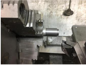
Here is a trial cut on steel. No visible chatter with a 0.002 inch deep cut which tells me the modified toolholder has not hurt my ability to take light cuts.
