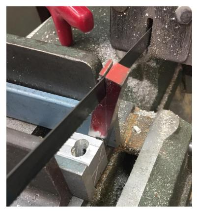
I then placed the blade back into its cut and clamped the part. You can see my blue extension jaws plus a small block of aluminum needed to secure the bar. In this position, the sawing went much faster than with the blade vertical and me pushing on the part.
