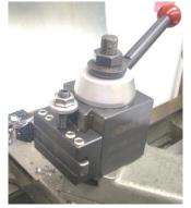
When using the Diamond Toolholder, I must unbolt the QCTP, turn it about 12° and then tighten the bolt. This puts the cutter at the correct angle for turning and facing.
