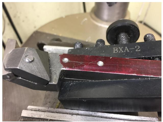
Time to match drill. The Diamond Toolholder, CRS bar, and the QCTH as an assembly was moved to my drill press. Using a digital protractor, I set the flank of the Diamond Toolholder level. Then I used my <sup>1</sup>/<sub>4</sub>" spotting drill to cut two cone shaped holes. The exact hole placement was not critical. I held up a 10-24 socket head screw to be sure nothing interfered.
