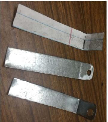
cut a paper model for my sheet metal strips. Since this was a proof of concept, I didn't waste time making the sheet metal precisely. The holes were eyeballed as was the width.
