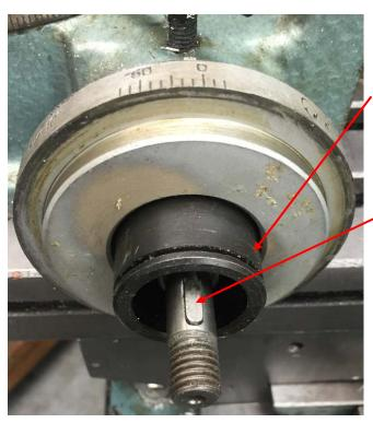
With the crank and dial removed, the driven shaft is exposed. It has a diameter of 12 mm. That black cylinder around it is 1.497 inches in diameter. It is solidly connected to the back dial disk.
