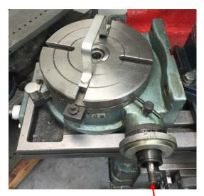
Many people have connected a stepper motor to a rotary table in order to perform the A axis function. I already had the rotary table. It was used on rare occasion but was still worth keeping. Once I went to CNC, its value decreased further. So it was a natural to turn this obsolete attachment into something useful.
