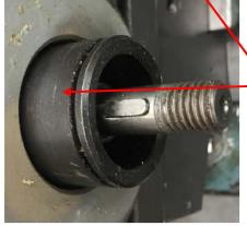
Set screws would be used to lock the support to the rotary table's black cylinder.
