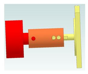
Initially I planned to have two set screws on the motor shaft and one set screw on the rotary table shaft. The internal key way that mates with the rotary table's key was a snug fit so I didn't bother adding a set screw on that end.
