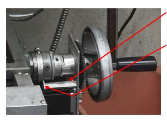
Paul used two cylinders flanking the drive shaft. One end of these cylinders bolted to a support plate for the gears and motor. The other end had L shaped brackets screwed in. The brackets were captured under a hose clamp. I know what you are thinking because that was my first impression too - how *cheesy*! But over time I grew to appreciate this elegant design.
