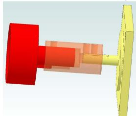
The coupler has been drawn in and made translucent so you can see how it mates with the rotary table shaft and the stepper motor shaft.
