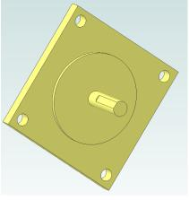
Then I drew a 3D model of the NEMA motor's important dimensions. The shaft is ½ inch in diameter and has a 1½ diameter boss around it.
