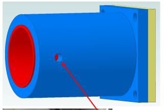
My initial design was massive. Cut from a single block of aluminum, it had a 1.5 inch inside bore and a flange on the end to match the motor. The cylindrical part had a wall thickness of 0.25 inches.
