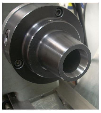
Here is my CDCO Machinery Corp 5C collet chuck. It has been carefully mounted on a semi-finished back plate that has been machined in place on my lathe. As I measure the face of this chuck and its outside diameter, you would think I did a fairly good job. But take a close look at the tapered bore. When I measure it, I get a TIR of 0.01". That sure is a far cry from the 0.0004" shown in the spec sheet.
