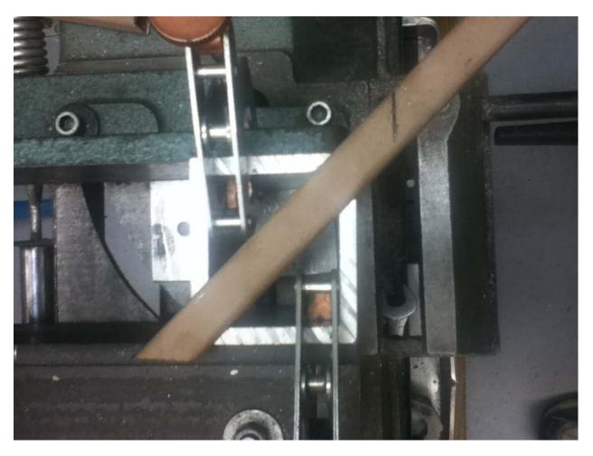
Sure I can unclamp my horizontal/vertical bandsaw jaws and set them to 45°. It is just a pain to do. And if I am making a series of 90° and 45° cuts, the pain is even greater. So instead I cobbled together a pair of softjaws that hold my square tubing at 45°.
