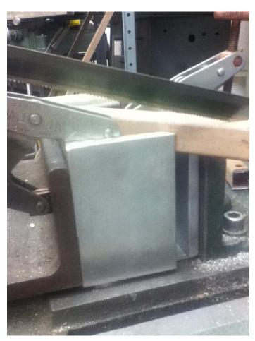
One essential element of this design that I failed to mention before is the left side stop. It is a piece of threaded rod that keeps the movable and fixed jaws at a given distance. This lets me clamp the tool on the right and not have the movable jaw pivot. You can see it disengaged in the next picture.
