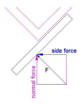
If the corner of the angle support is to the right of this force contact point, the side and normal forces cause the bar to pivot clockwise and not clamp.
