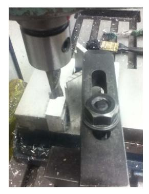
Here you see one of the softjaws being machined. On my first try I used just the force of the vise to hold it in place. The part lifted up slowly from the pull of the endmill and spoiled the cut. Oh well, turn it over and try again, with an added hold down clamp.
