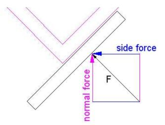
I think this is why. As I tighten the vise, the movable jaw moves closer to the right side face of the angle support shown in the last picture. But when there is contact, the applied force, F, is perpendicular to the bar being clamped. This force can be resolved into a side force and a normal force. I say "normal" because it is perpendicular, or normal, to the fixed
