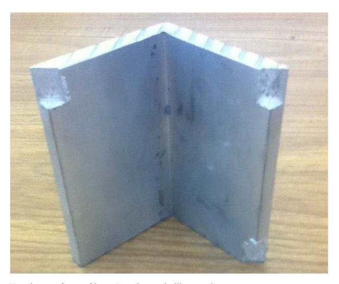
Here is one of my softjaws. I used an endmill to cut the steps on top outer corners. They are about 0.1" wide maximum and 0.4" from the top. This was a quick "proof of concept" job so admittedly it looks a bit ratty.
