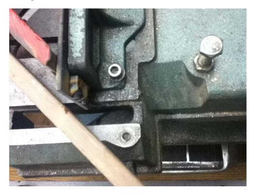
This chock prevents the angle support from sliding to the left as force is applied by the movable jaw. One problem here is that I must add packing between bar and angle in order to clear this chock. Moving the angle to the right and welding from the inside would avoid this problem.
