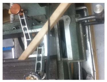
I did have to place a piece of scrap 1/8" aluminum plate under the softjaws to get the bottom of the steps above the top of the vise jaws. Other than that, the arrangement worked well and I quickly cut the 6 diagonal braces needed for my latest project.
