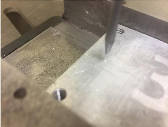
Here you see a faint scribed line with a punch centered on it. My spud is being positioned so the point enters the dimple.
