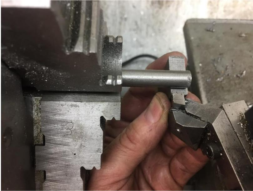
I'm going to be making a lot of 3/8" wide steps that do not have to be very precise. I chose a scrap of 3/8" thick stock to use as a gage. Just eye-ball the cutter's position before each step is cut. **NEVER** do this with the lathe running.
