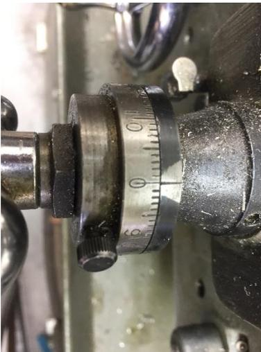
With the lathe running, feed in the cutter until it barely touches the stock. Then zero the in-feed dial.
