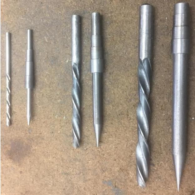
The spud to the far left is the same length as my 1/8" drill. It has a minimum diameter of 1/8" and a maximum diameter of 1/4" (0.125, 0.165, 0.205, 0.250).
