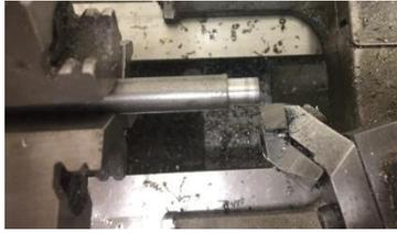
Repeat these three steps but this time the dial is at  $20 + 20 = 40$  thou. Our second step is done. The third step is the original outside diameter (OD) of the stock. If you like, take a light cut over this step to true it up.
