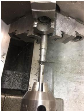
Without disturbing the part in the chuck, spot drill the end. A spotting drill has an end like a regular drill but the rest of the body is smooth. It is a good way to cut a cone shaped hole that will later center a drill.
