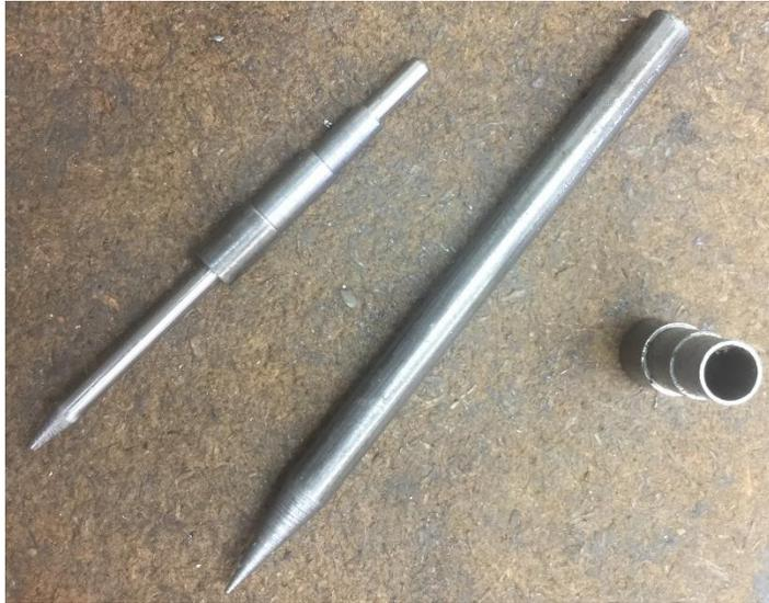
If you reamed the holes, the rods should be a snug sliding fit into the stepped collars. If drilled, they may slide a bit more freely. This will decrease accuracy a little but should be fine.
