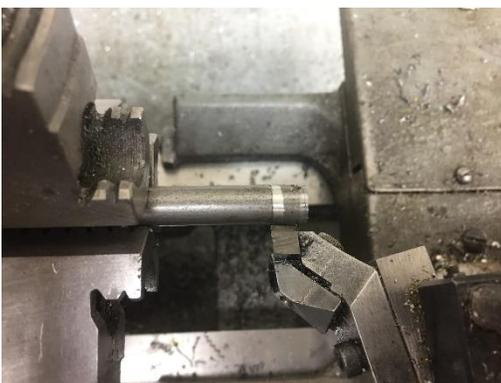
Next, feed in enough to cut a line to mark the step width.
