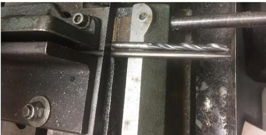
Next, take each rod over to your saw and cut them to the same length as your drill bit of the same diameter. Using a file or sander, smooth the cut end.
