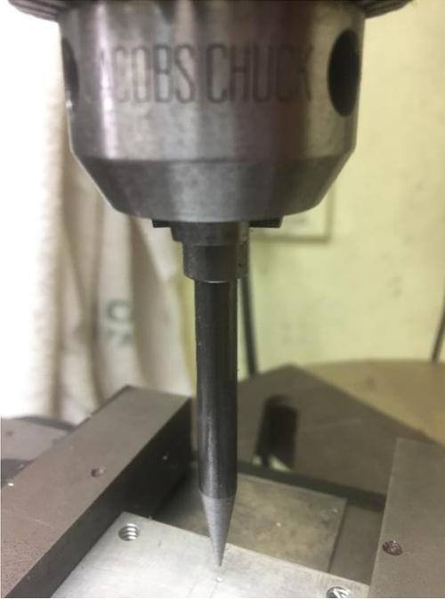
Grabbing the largest diameter, the end of the rod has bottomed out in the chuck. Yet there is enough contact between spud and chuck jaws so it is aligned.
