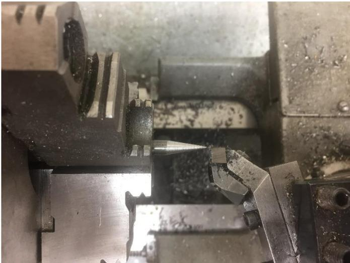
Start by checking that the cutter is right on the center of rotation so the point will be as sharp as possible.
