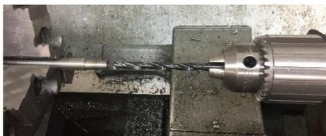
Next, drill the hole that will pass the pointed rod. If you have a reamer of the correct size, drill the hole about 0.01 inches undersized. If you do not have such a cutter, just drill the hole to size.
