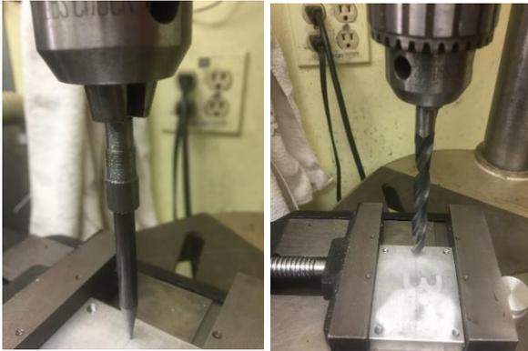
This Drill Location Tool is based on a pointer called a “spud”. I’m guessing that the name comes from the spud wrench:
