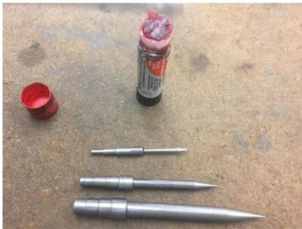
With a reamed hole, Loctite Red can be used to secure the parts. I prefer the gel rather than the liquid in this case.
