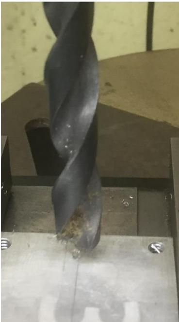
Then drill the hole nicely lined up with the punch mark. This picture shows how difficult it can be to even see the punch mark with the drill over it.
