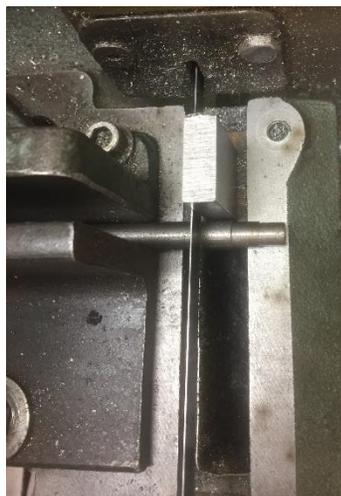
Saw off the part again using the 3/8 inch block to set that last step. Leave a little more width so the end can be trued up on the lathe. **NEVER** make these adjustments with the saw running.
