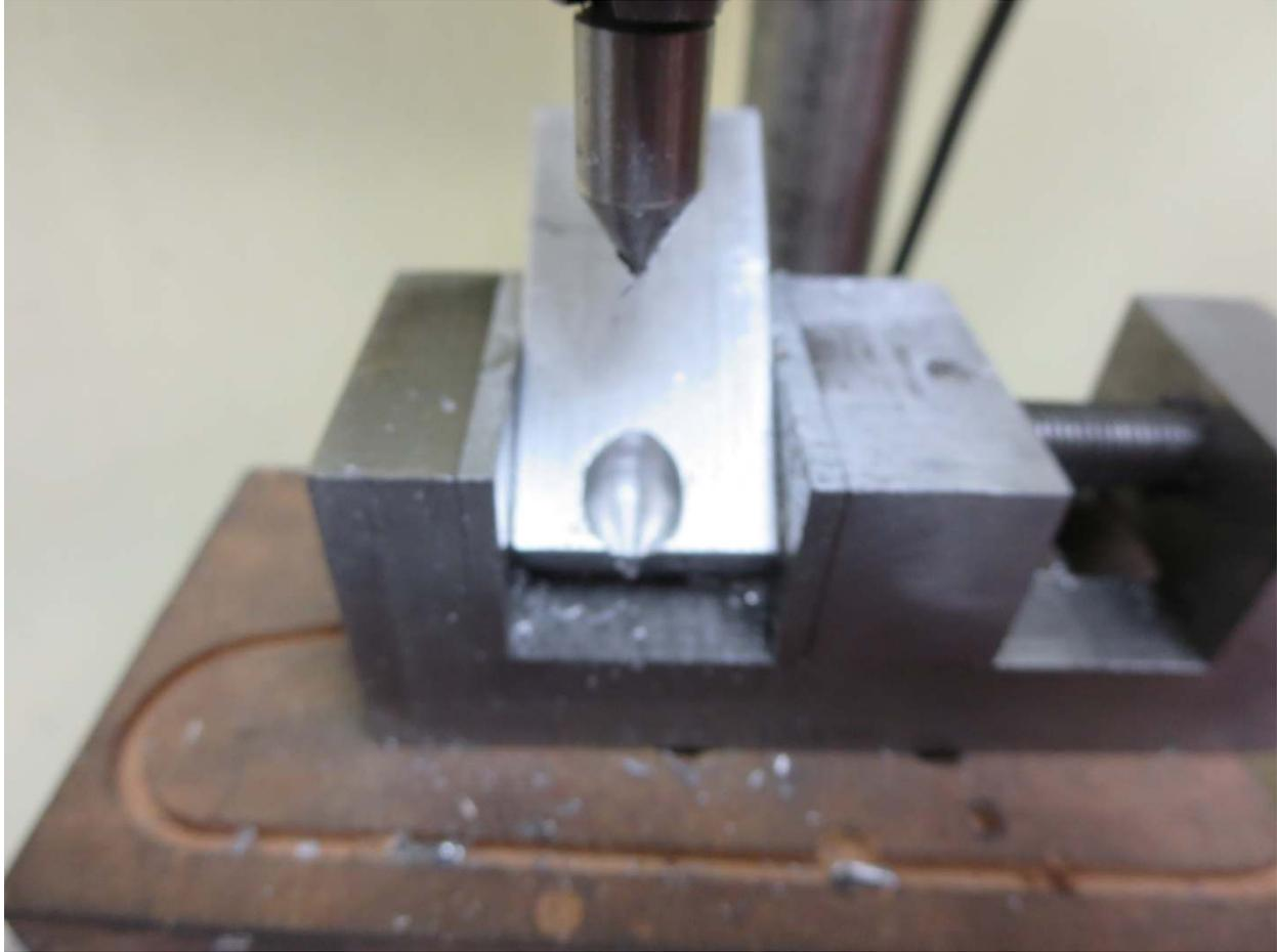
You can see that the bottom of the hole barely broke through the end of the workpiece. This was a bit too close for comfort. However, I still had milling to do in order to have the end of the block pass just beyond the center of the hole.
