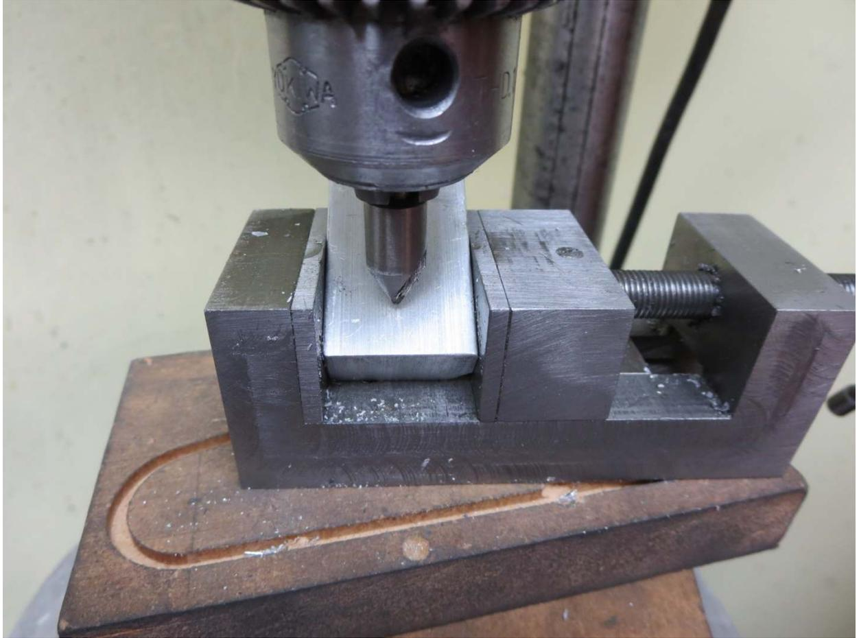
The hole was started far enough back from the edge of the workpiece so it did not break through the end.
