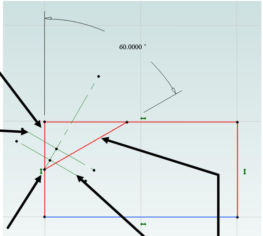
Say that this lower line, perpendicular to the centerline, is the end of a small diameter bolt. The right bottom corner of the bolt touches the right flank of the tapered hole. The left flank must be at the vertical face of the block.
