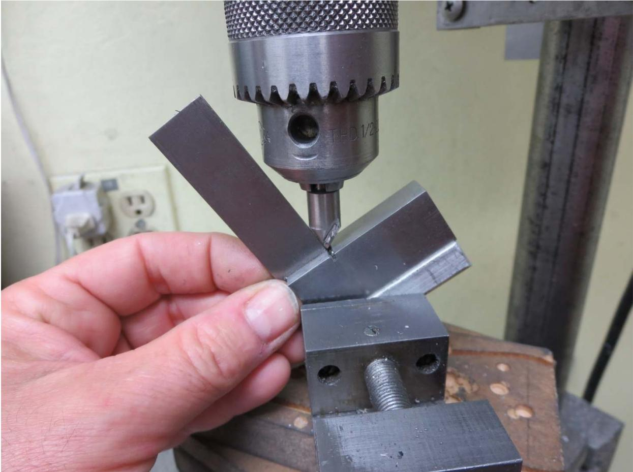
A 3/8" diameter 60° included angle countersink was mounted in my Gingery drill press. The workpiece was then clamped in my homemade vise. I used a 2" square to set the workpiece so the left flank of the countersink was perpendicular to the face.
