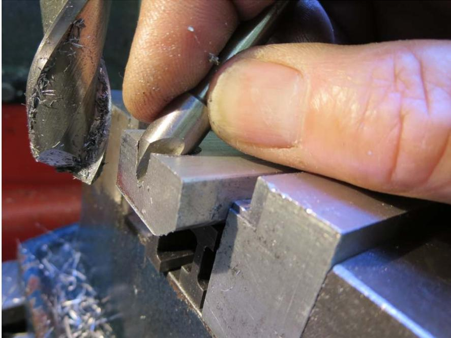
The fixture consists of drilling an angled hole in a piece of aluminum using a countersink. Then the end of the workpiece is milled off until the center of the hole is a little over the edge. The ideal location will be explained in the next section.
