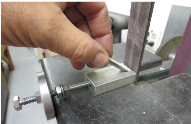
The last step was to drill and tap a hole in the end of the block to accept a long bolt. An arrangement of washers and scrap parts made up the stop.
