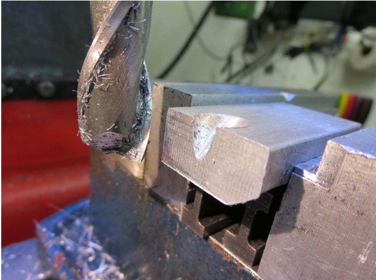
I ran the mill across the end of the work piece until just the center bottom of the hole was exposed. Then I used a 16 TPI bolt as a gage for the final cut as explained in the theory section.
