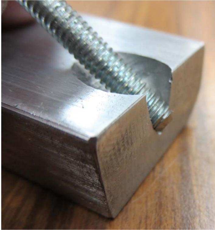
Here you see a 1/4-20 bolt in the hole. Note that the thread at the end of the bolt is exposed. When the end of the block is close to my sanding belt, a bevel is cut in the threads. The user must keep the bolt roughly centered in the hole and give it a full turn.
