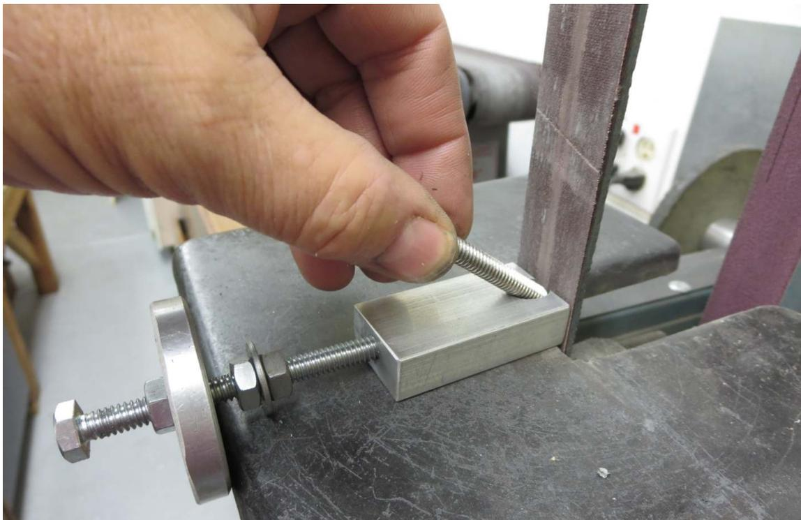
If you have built the Universal Bolt Cutting Fixture, there is a small pile of cut bolts waiting to have their ends beveled. The fixture presented here solves that problem. It can bevel any bolt from 3/8" on down to at least #6.
