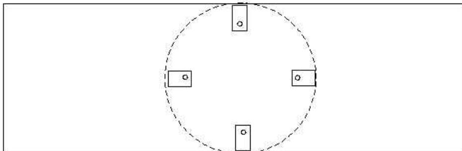
After taking a light cut over the top face of each pad<sup>1</sup>, I would place a dot with a black marker to define the exact location of my reference point. The dot would be as close to the dashed line circle as possible. Then, with the spindle at the center of the circle, I would begin my tramping process.
