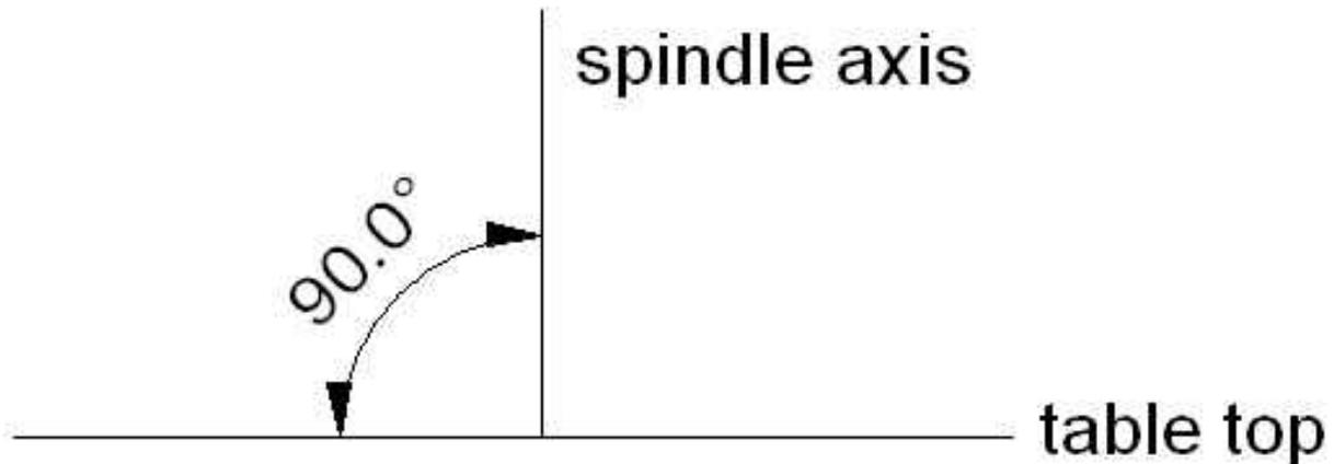
Assuming that the table top is flat, conventional thinking has it that the head is true when the spindle, or Z, axis, is perpendicular to the table top.
