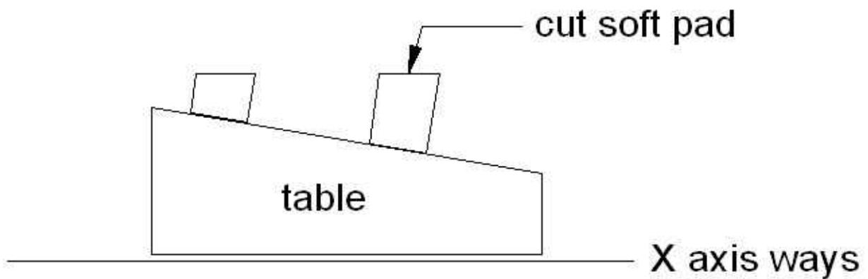
I then mill the tops flat. Even if the head is not trammed, I can get the tops of these pads arbitrarily flat by making each pass over the surface close to the last one. In the above example, we are only dealing in two dimensions so a single pass is sufficient. I now have the top face of each soft pad parallel to the X axis ways.
