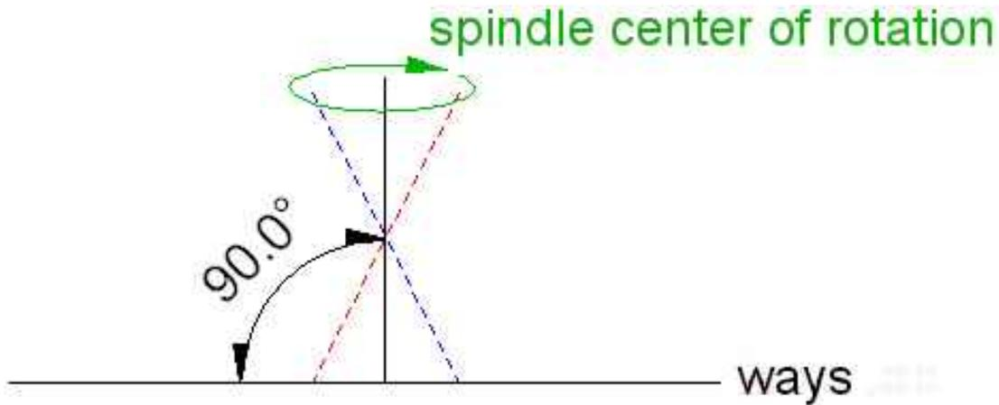
Ideally the center of rotation would be aligned with the Z axis. Rotation should not change its relationship to the ways. If the spindle center of rotation moves as it turns, then we must have this error.
