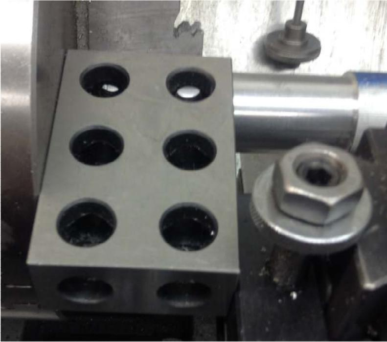
An elegant trick I learned when I got my QCTP is to place a 1-2-3 block on one of the jaws of the chuck. Then slide the QCTP's face into the block and tighten the top bolt. The QCTP is now parallel to the chuck face so perpendicular to the center of rotation.
