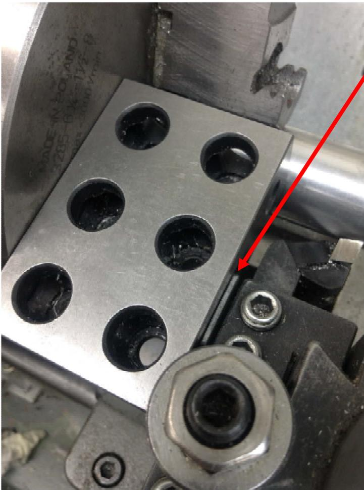
I loosened the center bolt on the QCTP, moved the QCTP such that the angular stop touches the 1-2-3 block, and tightened the center bolt.
