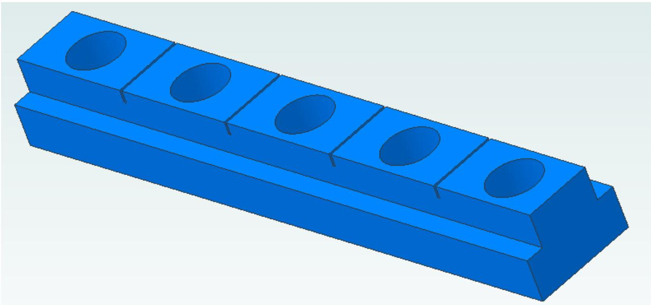
I could drill the hole in one pass but it would be rough on the drill and on my mill. Instead I "step drill", using a 1/4" drill and follow with the 27/64".
