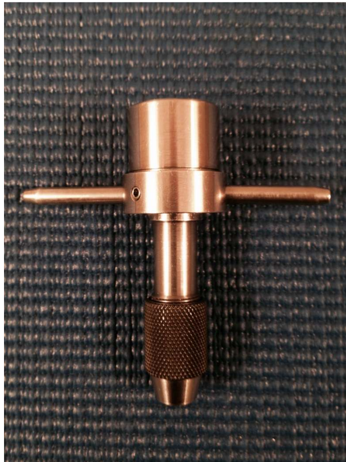
Figure 6: Starrett No. 93-A tap wrench held in stainless steel collar with set screws
