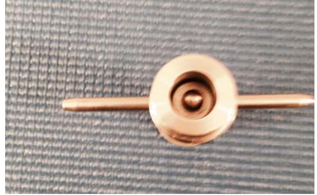
Figure 8: Collar recess with magnet inserted
