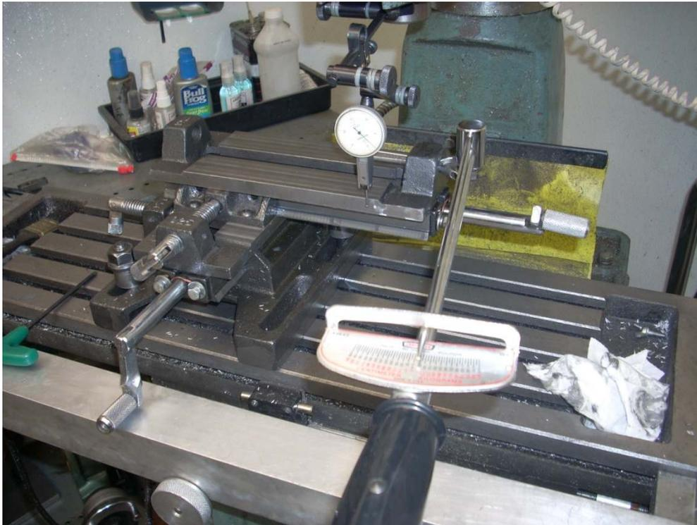
There are times when I see an error in my machining yet have no idea where it came from. Is some supporting member bending or is it not clamped tight enough? Such was the case recently after re-machining a Harbor Freight XY compound.
