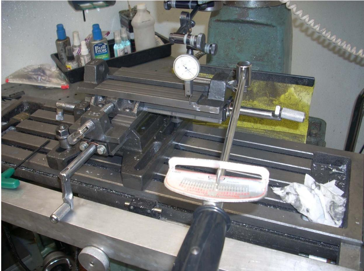
The procedure is rather simple. I move the mill table such that the DTI is at the center of the slide ways. Then the mill table is locked and I apply +200 inch pounds and then -200 inch pounds while watching the dial. The torque wrench fits into a small adjustable wrench that slides into a hole in the slider. This arrangement effectively couples my known torque into the table.
