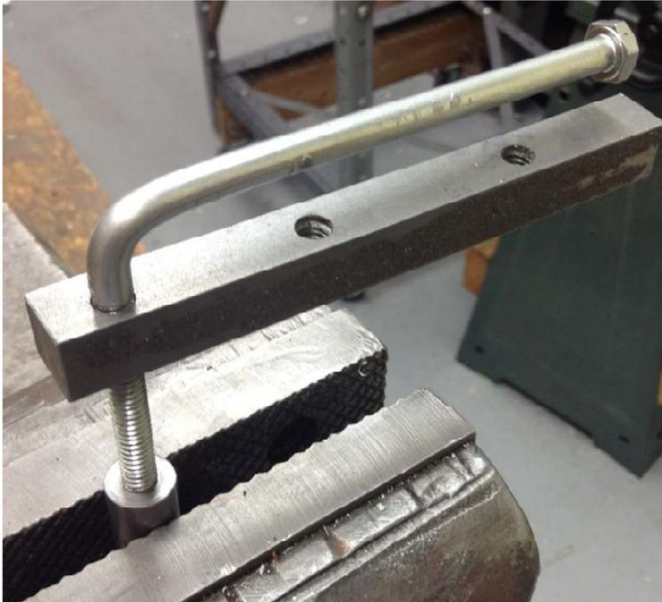
To drive in the stud, I first screw the body onto the stud. Either the end or center hole in the 1/2" bar can be used.
