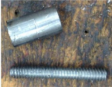
The cylinder has a blind hole tapped  $\frac{1}{4}$ -20. I want to screw the piece of threaded rod into it without damaging its threads. I did *not* want to take a long side trip to develop a handsome new tool at this time.
