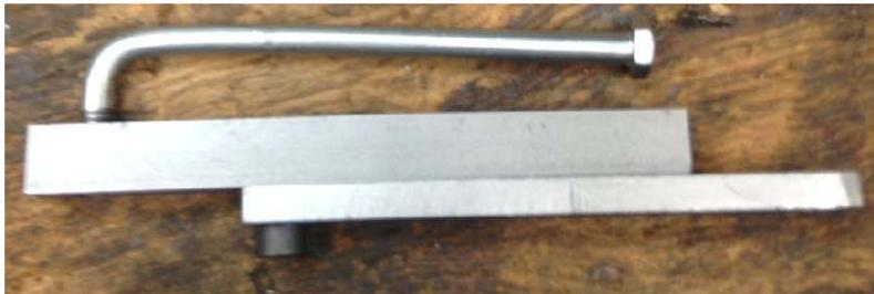
Here is my slapped together, "git 'er done" stud tool. It enables me to screw in  $\frac{1}{4}$ -20 studs without damaging the threads. It also lets me unscrew the stud in a similar fashion.
