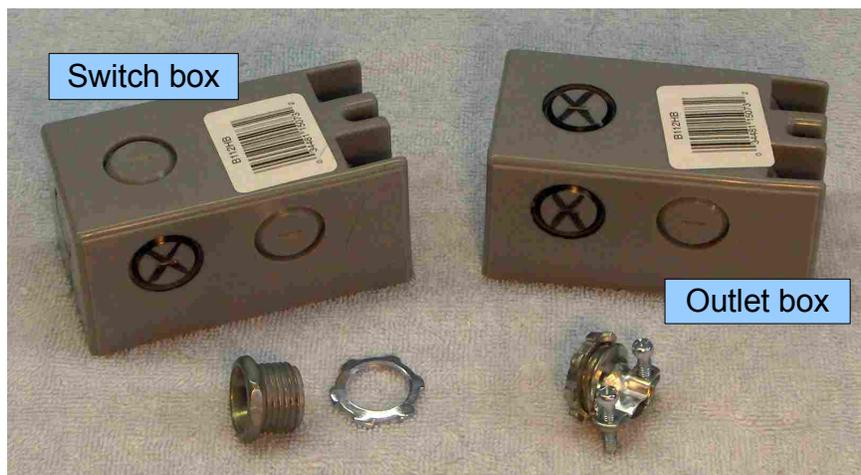
Assuming you want to mount the switch box at the right front of a tool, "surrounding" the corner as shown in the first photo, remove two of the knockouts (marked "X") from one box and one from the other. You can vary the configuration to fit your tool; remove whatever knockouts are appropriate. What you'll need, unless you're hard-wiring the switch, is a through-hole between the boxes and a power cord entry hole in one of them.
