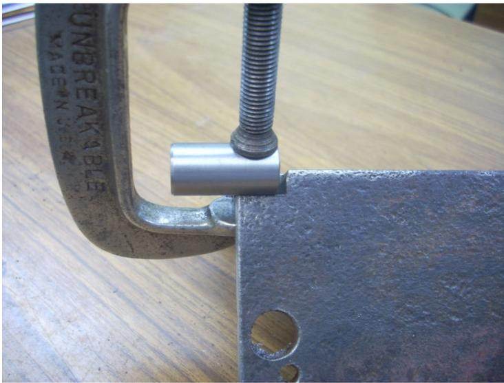
The resulting V accurately holds a short piece of  $\frac{1}{2}$ " rod as shown above. The C clamp is needed until I can weld the rod in place.
