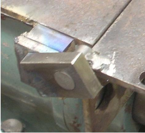
Here is a close up of the second hinge. I thought I had figured the width correctly but discovered that an additional  $\frac{1}{4}$ " of width was needed on the fixed part of the table. Not a problem – just tacked on a scrap of steel.
