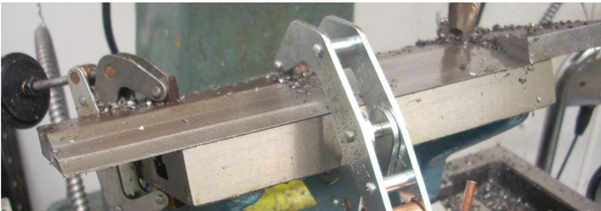
front clamp as needed to let the cutter pass. I was unable to mill all the way to the right end due to limitations in my X axis. I could have removed my vise and had room to shift the assembly over but that seemed like a lot of work.
