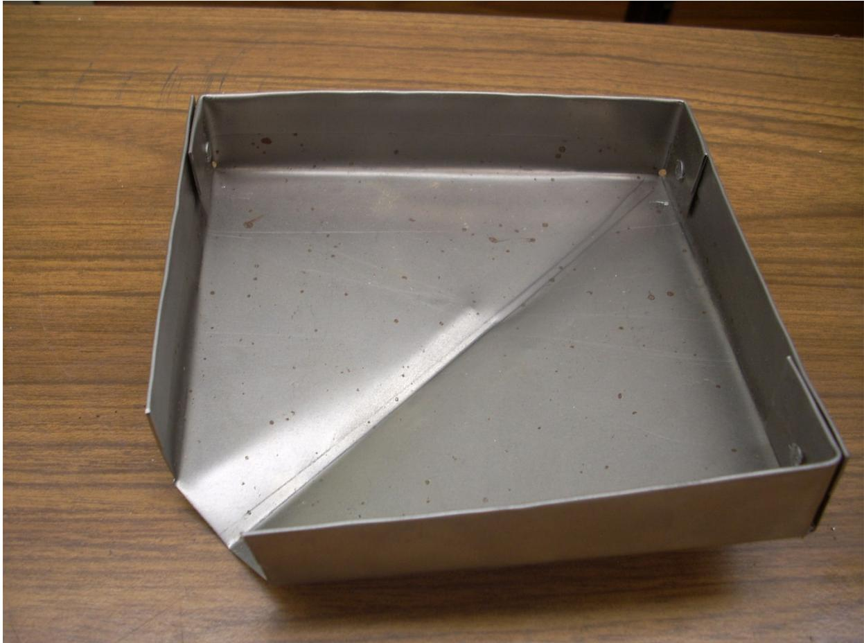
The inside of this tray is 5" so I used my 1" and 4" fingers for those bends. The open space flanking these fingers is room for the adjacent sides of the tray. One source for more information on how to use a finger brake is YouTube.com. Just search for "finger brake metal bending".
