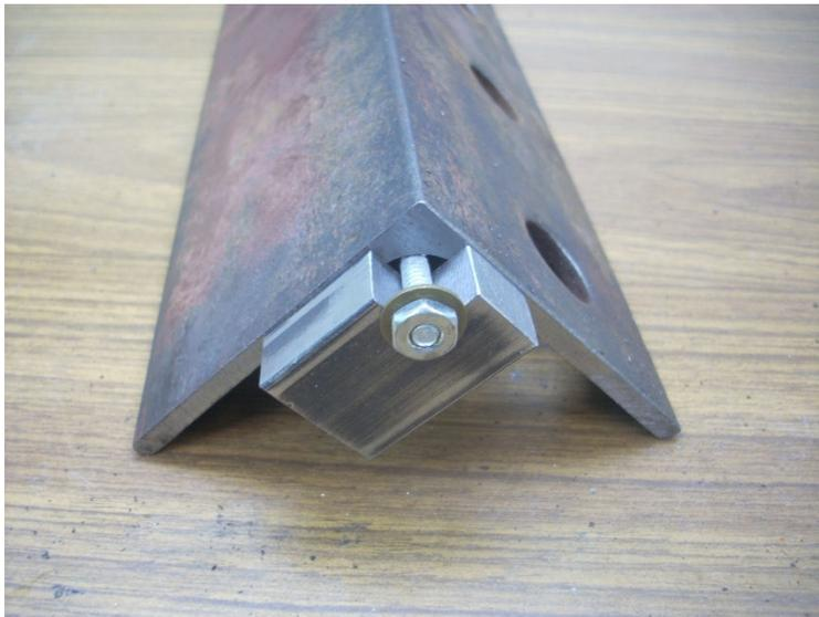
A length of threaded rod was used to hold these blocks in place until they could be welded. Note that the ends of the angle have been machined true. This is necessary in order to prevent binding of the hinge.
