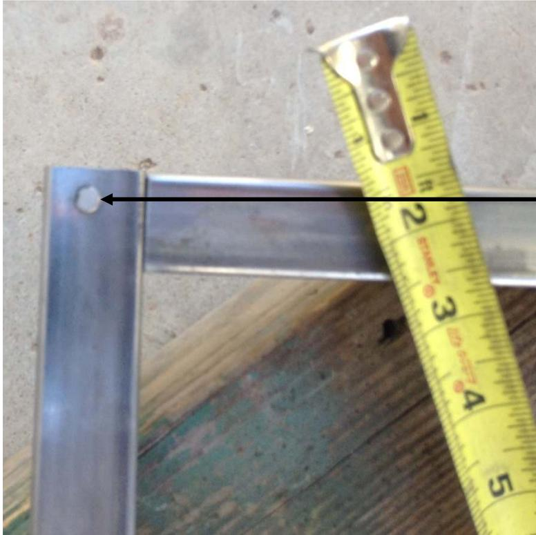
One annoying problem with measuring the diagonals is that the end of the tape measure does not always stay put.
