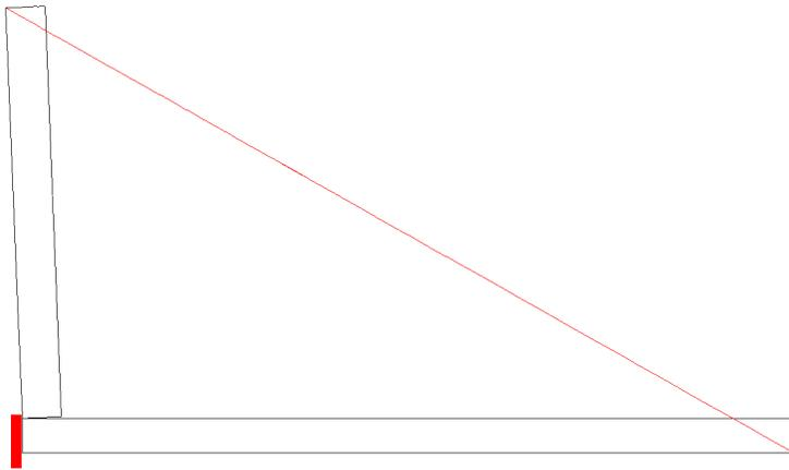
The corner is lightly clamped plus a stop is added to prevent misalignment. This might be a good place to use magnets.
