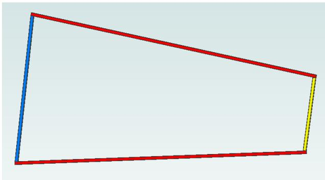
If you apply Rule 2 and adjust the frame until the diagonals are equal, you will make the two short sides parallel. But you will not have a rectangle.
