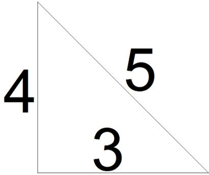
One way to solve this problem is to recall that a triangle with sides proportional to 3, 4, and 5 must be a right triangle.
