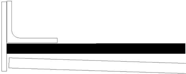
Especially when cutting long pieces, I clamp a piece of angle plus a plate to the end of my reference bar to act as a stop. It saves a bit of walking to verify the far ends are lined up. Do watch out for burrs that can prevent proper alignment.
