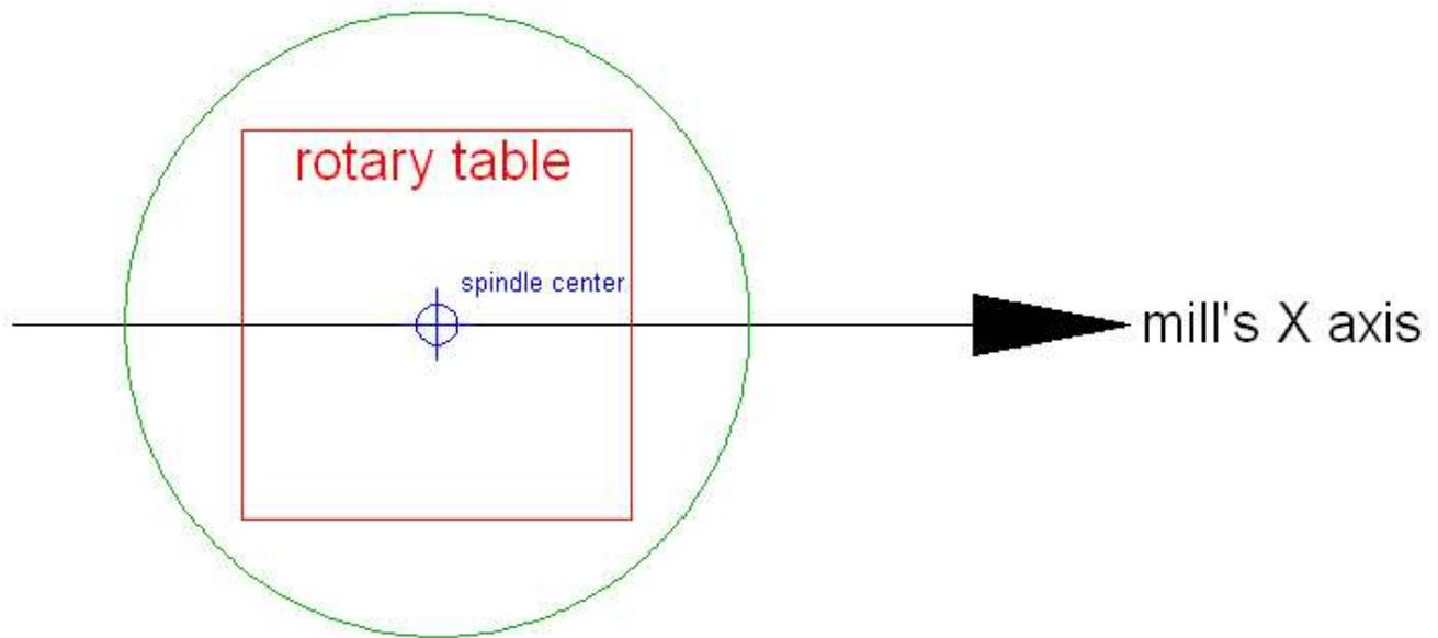
Now lets add the rotary table (RT). I have put the center of rotation of the RT at the spindle center.
