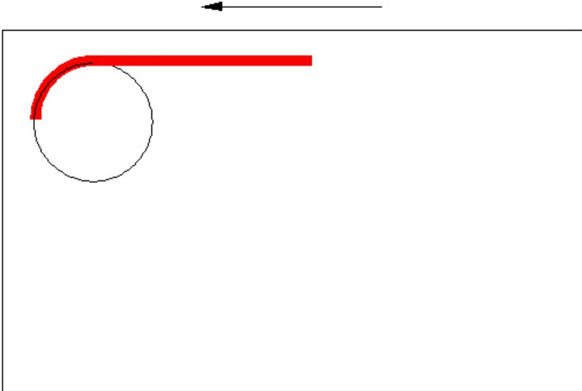
The RT X axis is now advanced as I cut the slot across the top<sup>3</sup>.
