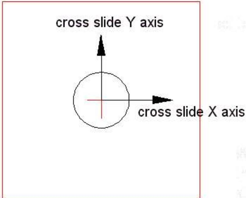
The cross slide is identical to the X and Y axes of the mill except smaller. Before it can be used in a sane manor, I must align it. We already went through the alignment of the spindle center to the RT center. The cross slide's X and Y axes must now be aligned. Typically a part is clamped to the cross side and some feature of it is defined as zero. When the RT X axis is aligned with the mill's X axis, I set zero degrees.
