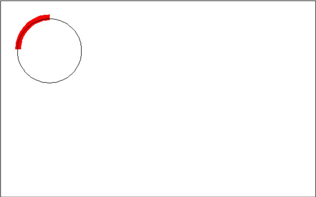
I will move the RT through  $90^\circ$  as I cut the arc. The fat red line represents the slot I have cut.
