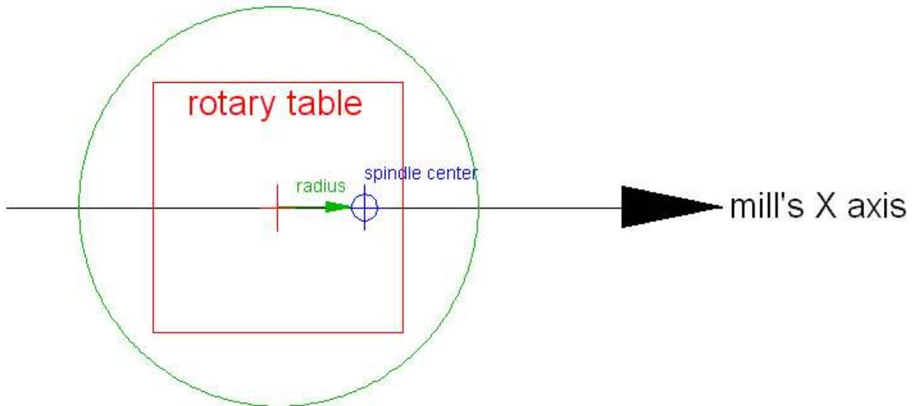
If I offset the RT center from the spindle center, a radius can be cut. Note that the radius shown above allows for the diameter of the end mill shown as a blue circle. The face of the end mill towards the RT center defines the inside edge of the radius. A second radius, not marked above, will exist that equals the inside radius plus the diameter of the end mill.
