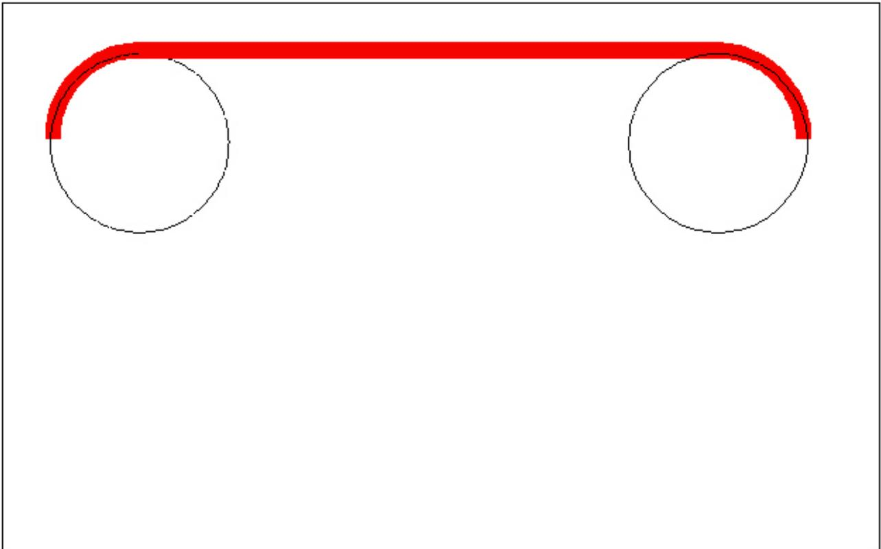
My RT is again rotated  $90^\circ$  and my second arc is done. The cycle repeats except this time I advance the RT Y axis. The lower right arc is then cut. The RT X axis is again turned until we are back at zero as the bottom slot is cut. One more arc to cut in the lower left corner. Then the RT Y axis is cranked back to zero and we are left with our slot.
