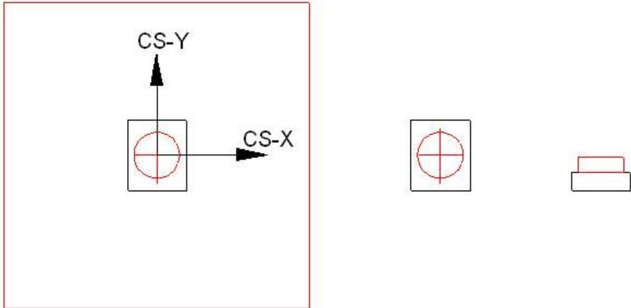
I have put a block down on the RT with its center defined as 0,0. The X axis was then moved to cut a radius. That was followed by milling away all material outside of the cut. I am left with a stud as you see above.
