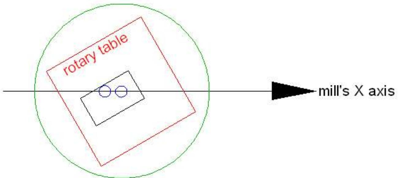
I have now rotated the block relative to the mill's X axis so my line of holes is no longer lined up with the edge of the block. It *is* still lined up with the mill's X axis and the hole will always be line up with the spindle's center.
