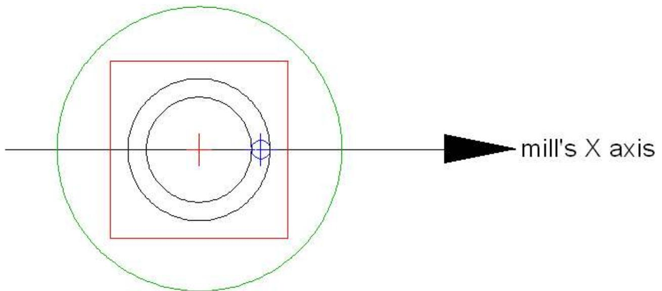
After turning the RT through the entire  $360^\circ$ , I get a slot with the two radii noted above. I can mill away the material inside the center of this slot and get a hole or mill out around the outer radius and get a round stud. I can also turn less than  $360^\circ$  and get many useful contours as you will see later.
