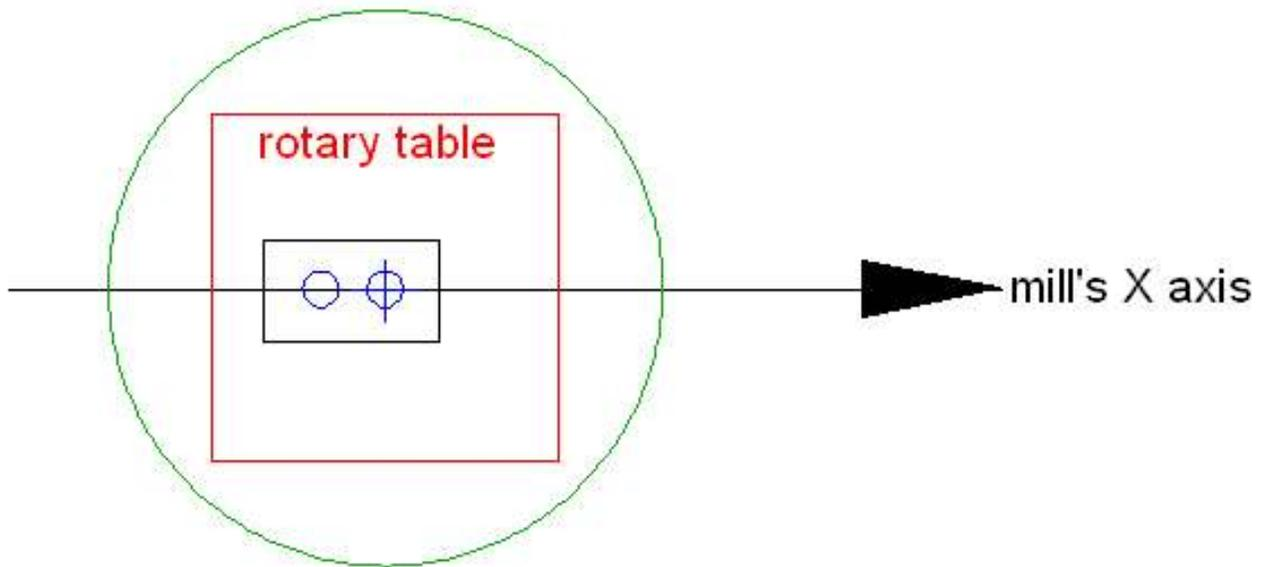
If I turned the X axis<sup>2</sup> feed of the mill, I would just get the same series of holes as shown without the RT. Not too exciting. What if I turn the rotary table first?
