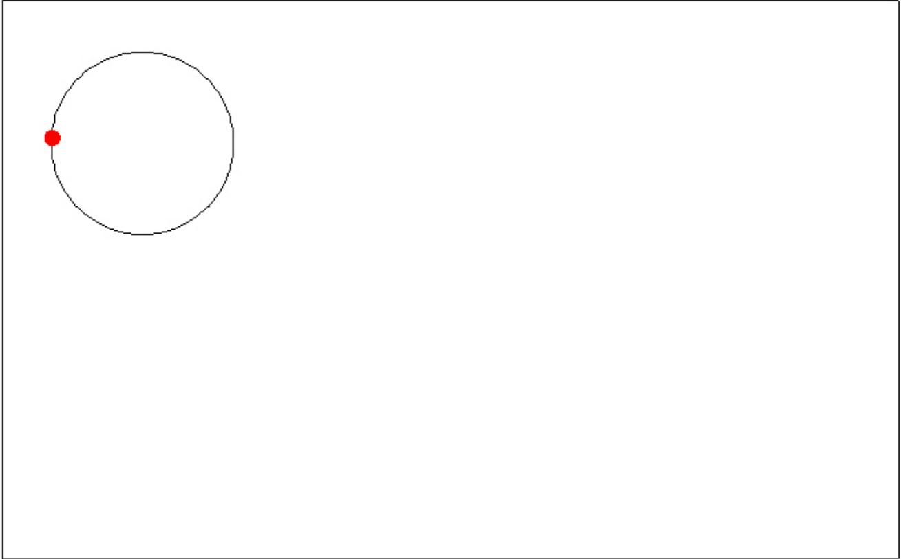
The red dot is the hole I will drill with the end mill. The black circle is the center line of the slot I would get if I turned the RT through a full  $360^\circ$ .
