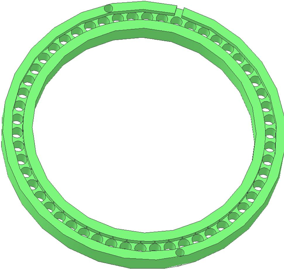
The ring was machined from nylon. There are 54 holes drilled with a #10 drill spaced equally around the bore. I originally planned to use a ring  $3/8$ " thick but the piece I found in my scrap pile was 0.6" thick. This let me cut my channel a lot deeper and made it easy to put all resistors and connections inside. I then used heat glue to pot it all after testing.
