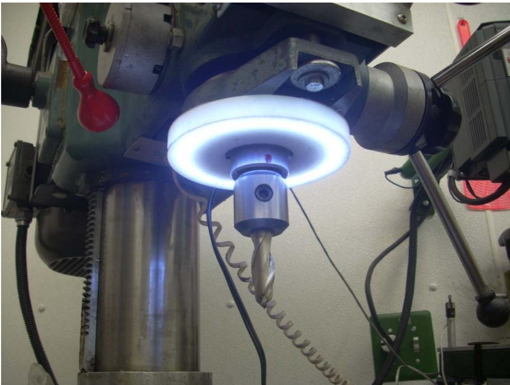
The ring was press fit onto the lower spindle bearing in this picture but I will add two screws into the bearing support very soon.
