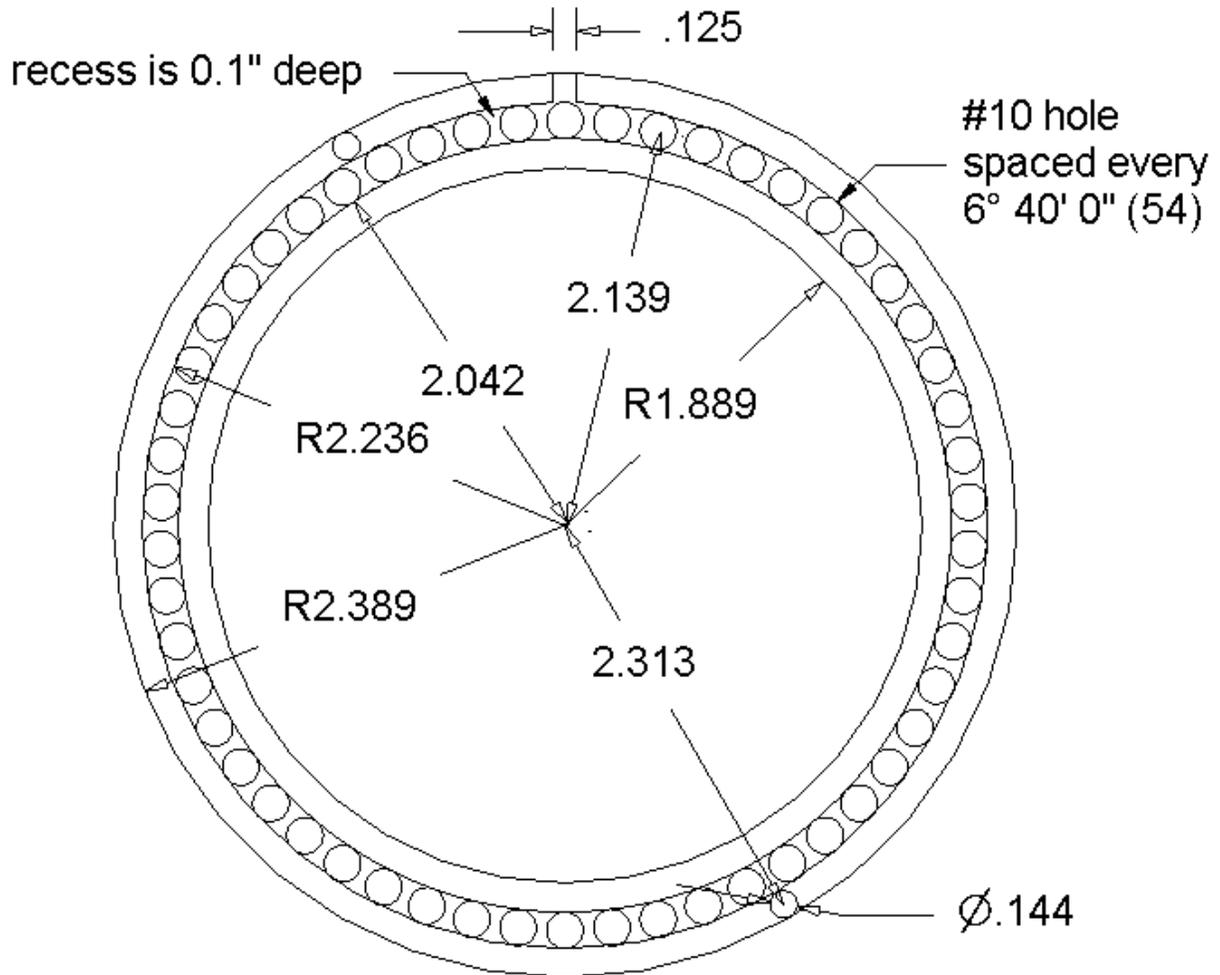
Ring holds 54 LEDs. The LEDs are grouped in sets of 9 in series with one 470 ohm resistor. All 6 strings are in parallel and powered by a 35V wall wart. Total current drain is about 100 mA
