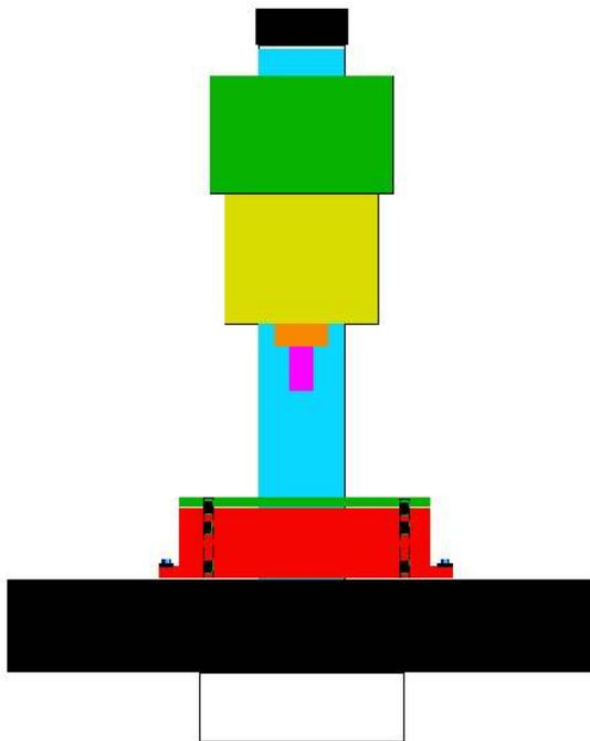
My zero height position is with the top plate fit into the base. To raise up 1", add the 1" thick tooling plate with pins between them. For 2", replace that 1" plate with the 2" plate. For 3", use both of them. If more height is needed, make a 4" thick plate. That will get you from 0" to 7" in 1" steps.
