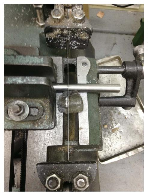
The first step was to cut off a  $2\frac{1}{2}$ " long piece of the drill rod. I used a chunk of paraffin wax as my cutting "fluid".
