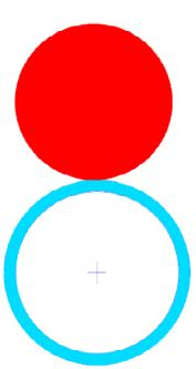
Next I moved the end mill to behind the workpiece and just touched down. Then I set my Y axis to zero.
