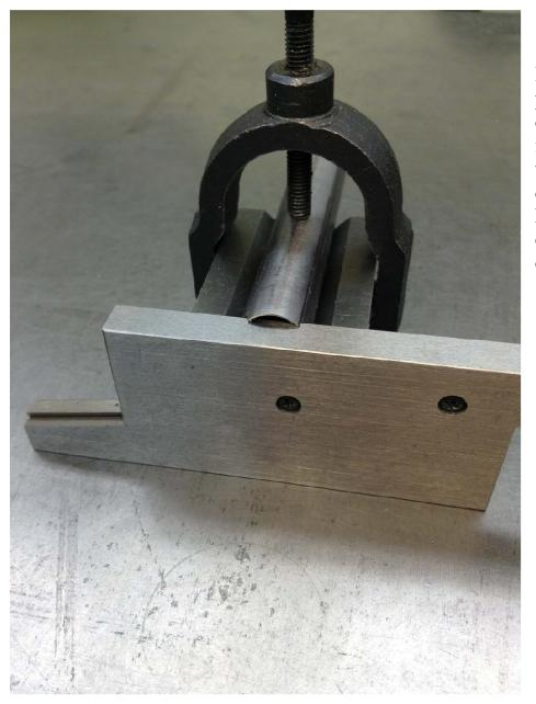
I used an adjustable parallel under the lip of the punch to align it on my V block. I was then ready to drill my set screw hole and have it centered on this cutting edge.
