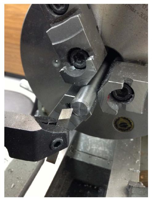
With the workpiece mounted in my 3 jaw chuck, I squared up the end and cut the bevel. The bevel looks nice plus prevents the top from mushrooming out from hammer blows.
