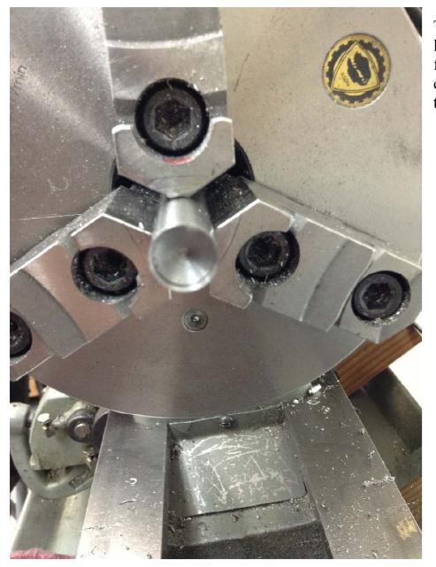
The result looked like this. I had formed a cutting edge with a uniform thickness at is root.
