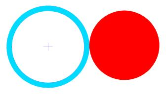
On the far left is an end view of the partially finished cutter. The blue is the cutting edge. On the right is the end mill. I started, with the machine off, by touching the end mill to the side of the workpiece. I then set my X axis to zero.
