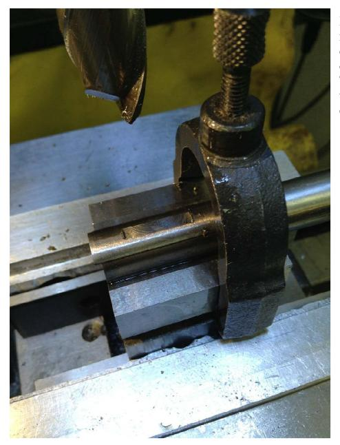
I still had my end mill mounted so first cut a flat in the flank of the workpiece. This made it easier to verify I was on center.
