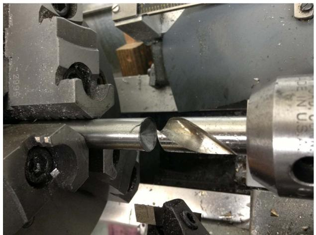
Next I used a  $\frac{1}{2}$ " spotting drill to shape my cutting edge. Just feed in until there is no flat on the end of the stock. Not shown in the picture is the liberal use of cutting oil.
