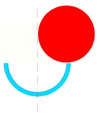
The end mill was then moved along the X axis until it's left face was about 0.01" from the red center line shown here. The end mill's Z axis was raised up so the depth of cut was back to a roughing cut, 0.04" from zero. I then started the mill and feed along the Y axis to remove half of the remaining lip. The end mill was then fed along the X axis to be right on the center line and advanced down the Z axis to a depth of 0.05" to perform my finish cut.
