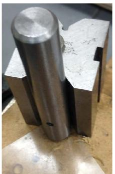
Here is the finished punch placed up against a V block. The V block performs two functions. First, it aligns the corner of the plastic directly below the punch. And second, it holds the punch in the right position.
