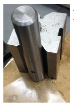
Then the punch was placed in the V. A quick tap with a ball peen hammer is all it takes.
