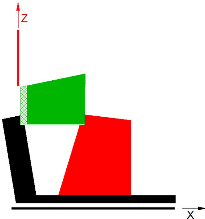
When I cut this top edge, it will be parallel to the X axis and perpendicular to the Z axis.
