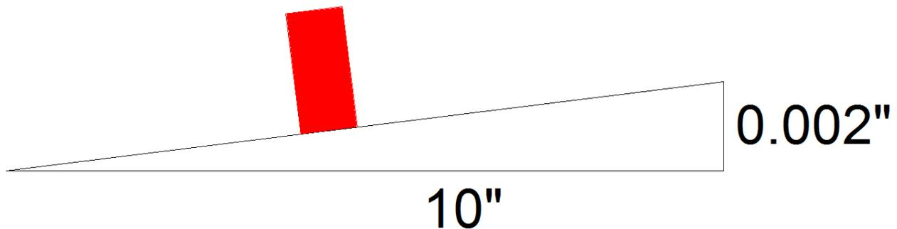
The face cut by side milling will have this same error. If the face was 1" tall, the error would be 0.0002. Even if you were able to side mill using a 10" long end mill, the error due to being out of tram would only be 0.002". This assumes that the end mill would not be bending due to the force of side milling.
