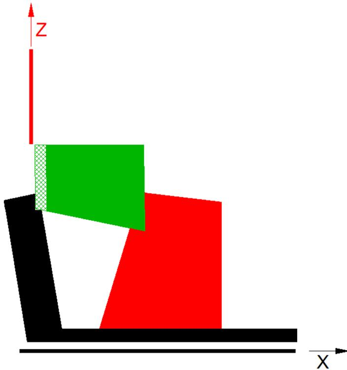
When I make my cut, I will get the top edge parallel to the X axis and perpendicular to the cross hatched edge.
