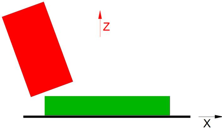
Back to our two dimensional view of the world. My end mill is not parallel to the Z axis but it still moves parallel to the X axis. As I cut the top of my green rectangle, I will still get a line parallel to the X axis. It doesn't matter that the end mill is off, I still get a line that is true.
