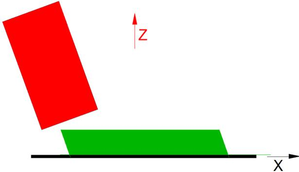
The place we run into trouble is when side milling. You can see the sides of my work piece are parallel to the end mill and not to the Z axis.
