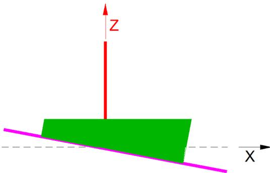
As I move my table, the top of the work piece is cut off. Note that the top of the work piece has been cut parallel to the X axis while its height varies.
