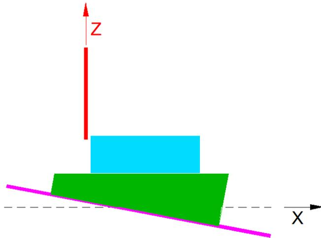
I plunk down a new work piece to cut. It is sitting on top of the green base that just had its top cut parallel to the X axis. Look familiar? It is the same as when we cut our first work piece on an ideal table.
