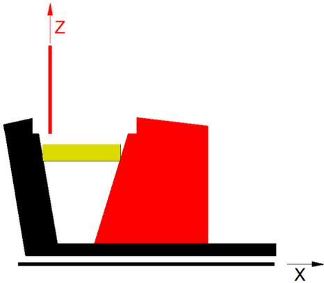
and will cut my soft jaws. To do this I first clamp a piece of packing in the jaws so that the vertical parts of the steps about to be cut are approximately the same distance apart as when I clamp my work piece<sup>2</sup>. Then I lock my end mill's height above the vise ways. Since this is just a two dimensional view, cutting involves moving the end mill left and right to cut the two steps.
