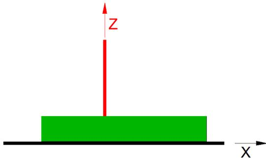
The green rectangle is a product of my ideal two dimensional milling machine. The top line was cut by the end of the end mill so is perfectly parallel to the X axis. The ends were side milled so are perfectly parallel to the Z axis.
