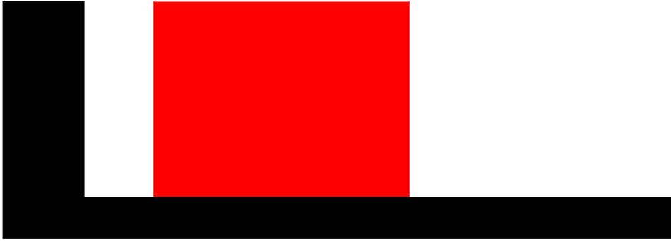
I have drawn a two dimensional mill vise. The fixed jaw and vise ways are black. The movable jaw is red.
