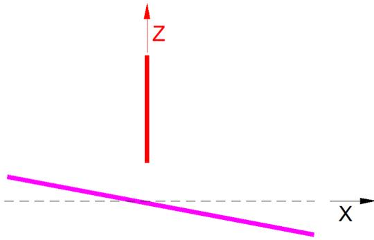
Let's now move one step away from this ideal case. My mill table will still be perfectly flat but it is no longer parallel to the X axis. However, my end mill is still parallel to the Z axis and the end of the end mill is still parallel to the X axis. My table still moves parallel to the X axis.
