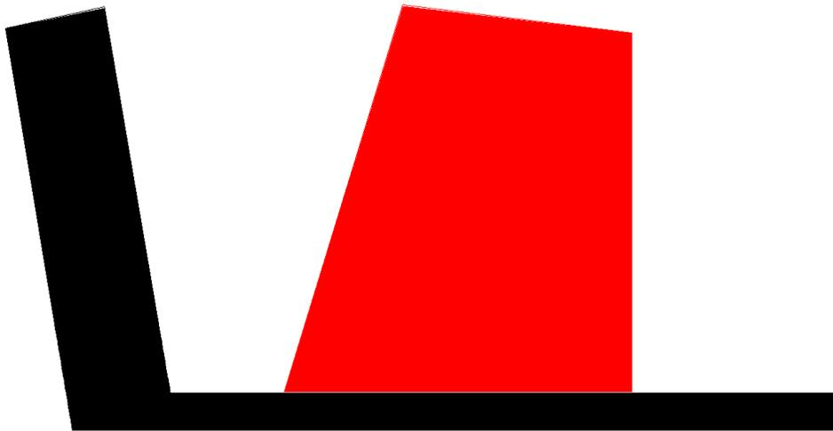
Contrast the above ideal vise with this sorry excuse. The fixed jaw and movable jaw are clearly not perpendicular to the vise ways.
