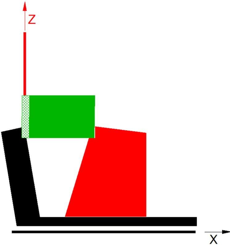
With the top edge cut, I now have a work piece cut on 3 sides. Each side is perpendicular to its neighbor. The 4th side is our reference and was already straight so did not need cutting.
