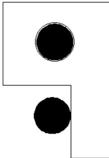
A variation on this idea is to replace the lower hole with a surface. As long as the slide block contacts the lower rod, the two rods do not have to be parallel.
