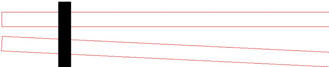
Say I bore a second hole in the block and fit a second rod. If this new hole is "much" larger than the rod, then the rods do not have to be parallel yet the block can move along the rods. The tighter the fit between new hole and its rod, the closer to parallel must be the rods.
