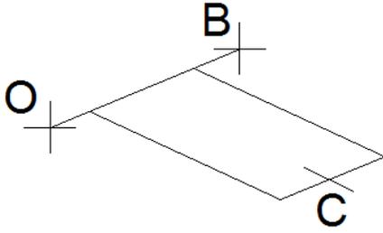
In the full 3 dimensional situation, the circles are hardened ball bearings resting on hardened pads. The balls fit into threaded rods that enable me to change the length of each leg while the ball stays on its pad.
