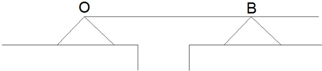
Point O anchors the bridge at one end. On the other shore I have point B. The bridge is a steel structure so will expand and contract as a function of temperature. Say the bridge is installed during the summer and is locked to its support at point B. As long as the temperature doesn't change, the length of the bridge between anchor points will exactly equal the distance between O and B.
