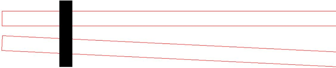
There are ways to side step this over constraint. The simplest way is to eliminate the second bar. The block will slide on the top bar and cannot bind up. That is not always sufficient.
