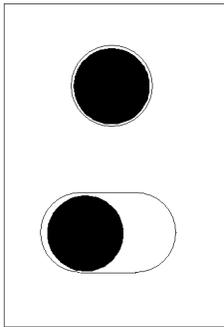
If the design requires that the block not rotate "too much" , it might be possible to have the second rod fit into a *slightly* elongated hole. This is a side view of the block. The wider the hole for the lower rod, the less stringent the alignment of the rods.
