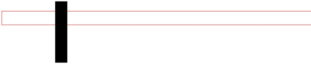
The red box is the outline of a precision rod. Assume it is perfectly straight and round. The black box is the outline of a block with a hole in it. The diameter of the hole in the block is equal to the diameter of the rod. OK, OK. The hole is a tiny bit larger so the block can move along the rod.
