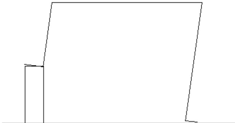
By using shims, I can jack up one leg and get the plate parallel to the reference surface. A single point is in contact between each flange and its supporting surface.
