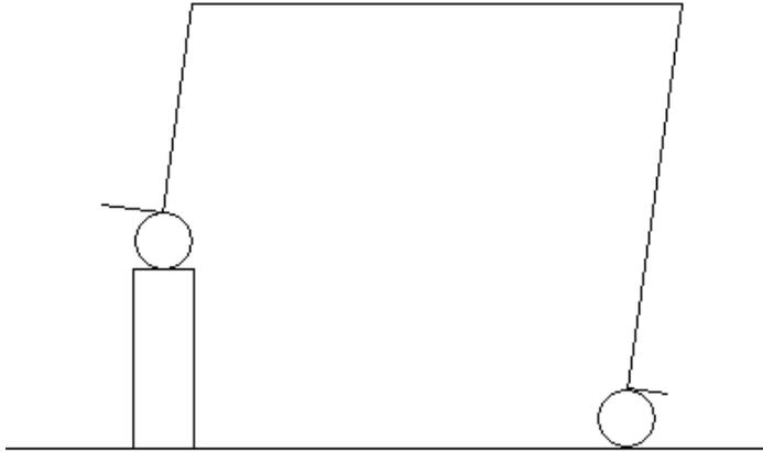
An elegant solution to this problem was given to me by John Herrmann. It involves placing a circle directly under each support leg. This insures a single point of contact. No distortion is possible because one and only one point of contact can exist between circle and reference surface.
