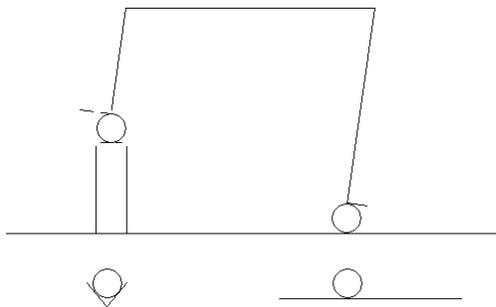
In order to insure reproducible positioning, the circle on the left fits into a V. This permits the associated leg to pivot but not move away from this point on the reference surface. The circle on the right fits into a groove (sides not shown here). This permits this circle to move left and right but not in and out of the page.
