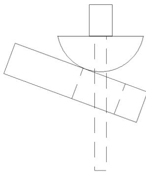
A hold down bolt is then run through the flange, past the circle, and into the reference surface. The bolt feeds through a cylinder cut into a D cross section. The hole in the flange is oversized. In this way, the bolt can pull straight down into the reference surface yet apply pressure to the flange. The cut cylinder is rotated such that it sits flat on the flange.
