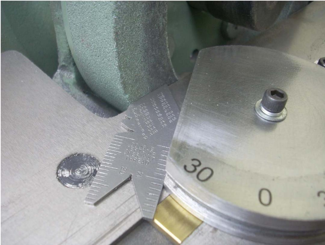
The exact angle should be set with a gage pressed up against the grinding wheel and the flank of the compound.
