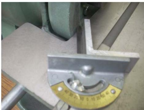
Now, if I put the cutter on end and support it with a right angle, I can get to +/- 60° by setting the compound at +/- 30°.
