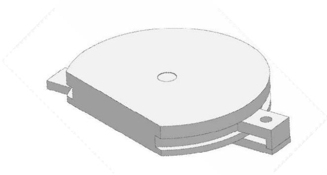
The tool support is made from four parts: the slider, the pivot, the clamp, and the compound. Not shown are two 8-32 Socket Head Cap Screws.
