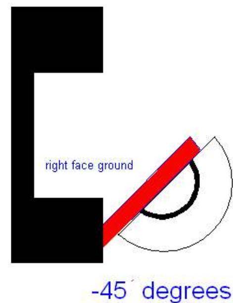
I can swing the compound over to  $-45^\circ$  and cut on the right side of the cutter. It cannot be turned more than this.
