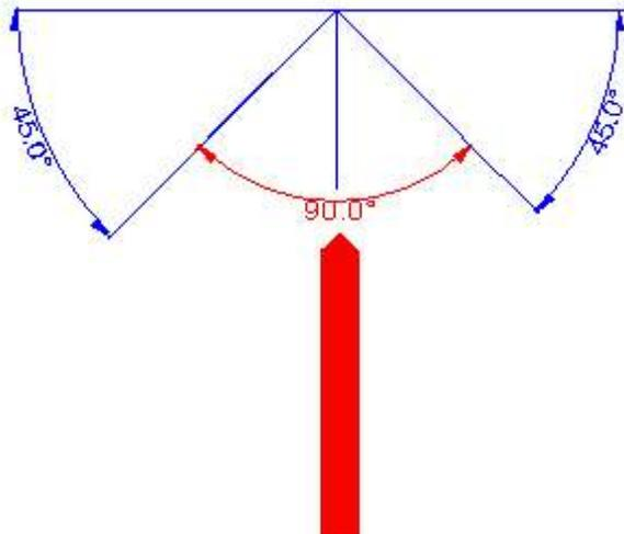
The resulting cutter has an included angle of  $90^\circ$ . Note that the compound's angle is measured from a line perpendicular to the center line of the cutter blank. Yet we usually talk about the angles on a cutter with respect to this center line.
