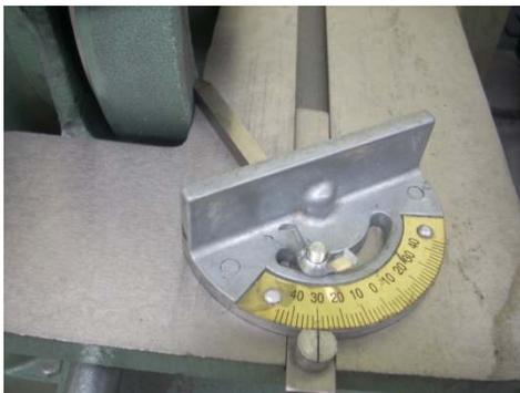
The tool support that came with my 1/2 HP 6" Tool Grinder enables me to grind any included angle from 90° to 180°<sup>2</sup>. That means that shaping a thread cutter with an included angle of 60° is a problem. I need to put this type of cutter perpendicular to the compound. Then I can grind any included angle from 0° to 90°.
