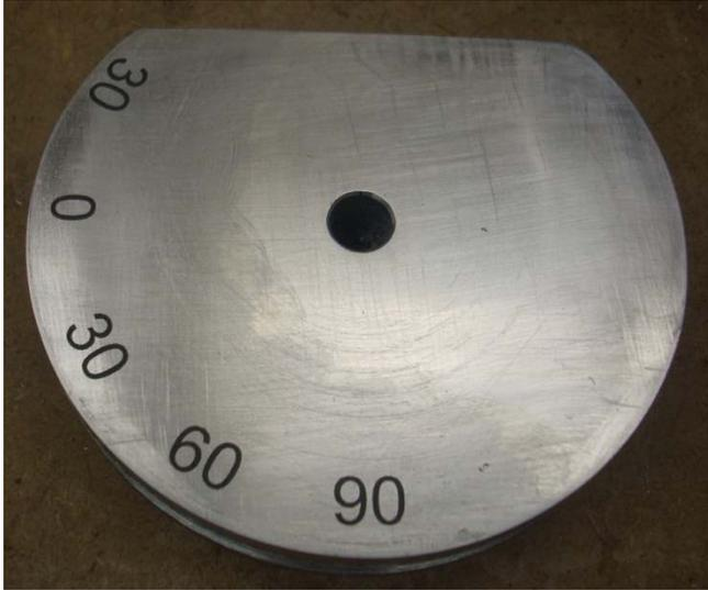
With the glue fully cured, I spray down a few coats of Rust-Oleum Crystal Clear Enamel Spray<sup>®</sup>. The solvent slightly melts the toner and darkens it. The enamel protects the toner.
