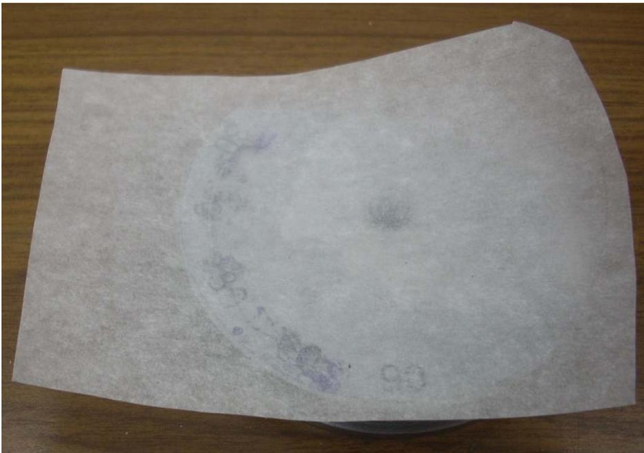
After coating the surface of the compound with Loctite<sup>®</sup> Glass Glue, I put down the mirror image artwork. It then set for about fifteen seconds before the paper lifts off. The Parchment Paper lightly holds the toner and the glue holds it firmly.
