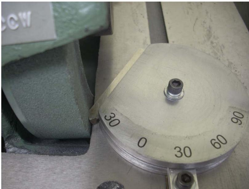
I grind the other face of the cutter with the compound set to  $+30^\circ$  and flip the base around so the clamp is in front.
