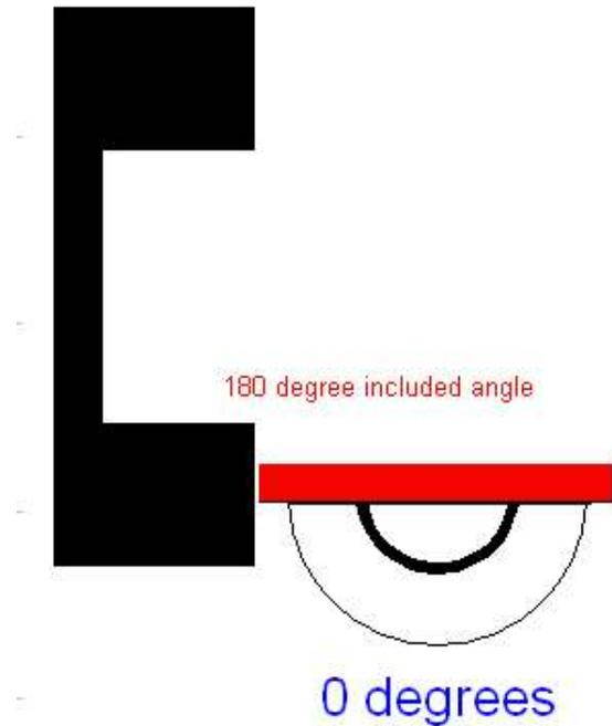
With the compound set to  $0^\circ$ , the cutter blank has the end ground square. This is an included angle of  $180^\circ$  as will hopefully become apparent soon.
