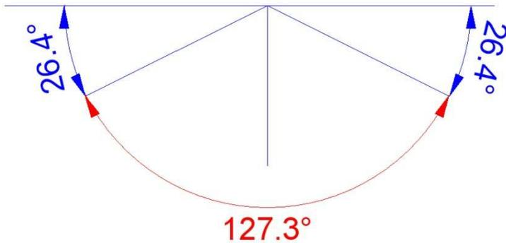
If I turned the compound to 26.4° and ground both sides of the cutter, I would get an included angle of
