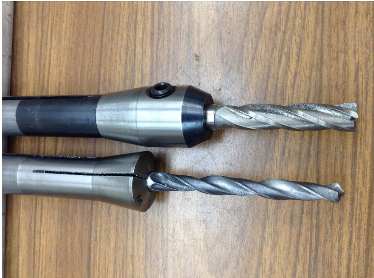
Since this happens to be a 3/8" diameter drill, I can hold it in one of the few R-8 collets in my collection. The end mill is now slightly *longer* than the drill. I might even be able to go back to my original end mill.
