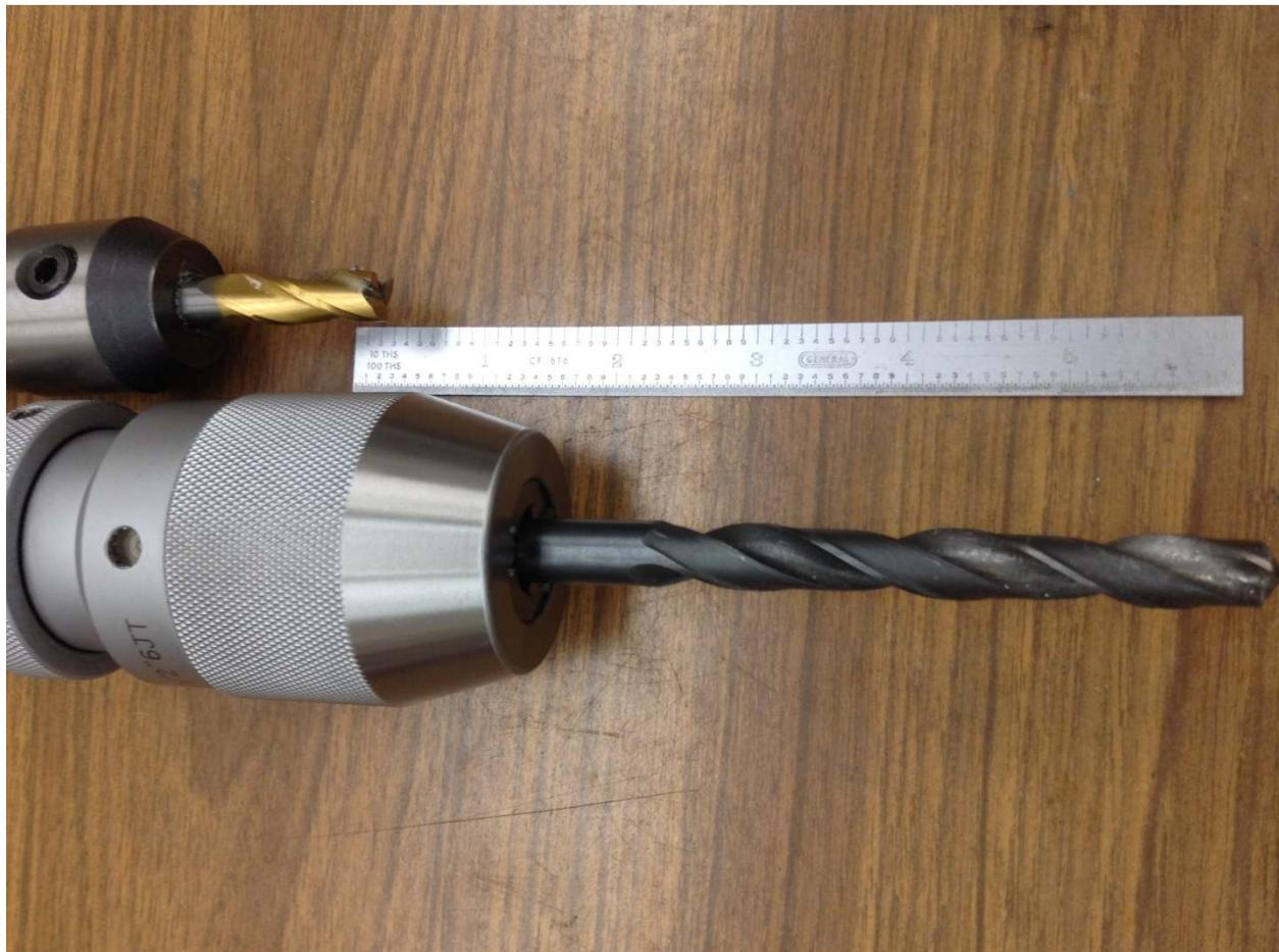
Here you see a typical dilemma. I have a 3/8" drill mounted in my keyless chuck and my 3/8" end mill. With their R-8 tapers lined up, you can see that there is more than a six inch distance between ends. If the head was set to be one inch from the bottom of the end mill, it would be impossible to even mount the drill chuck.
