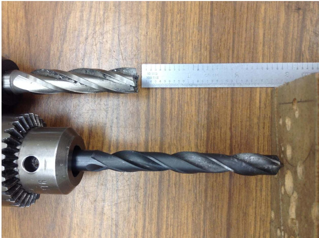
Maybe I can get the job done with a longer end mill. This end mill will deflect more than the original so I might have to take lighter cuts. The diameter is also larger which might not work. I've got one more trick up my sleeve.
