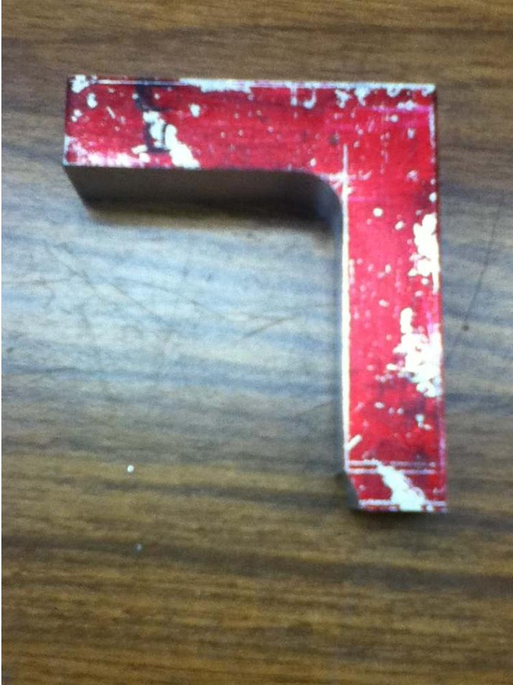
I removed the part from the mill in preparation for final deburring.
