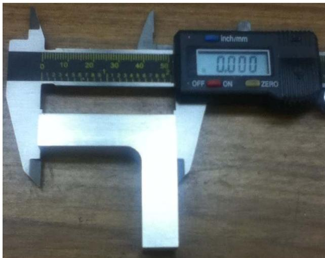
After deburring, I did a final check with the caliper. Now, that's a lot closer than being 0.251" off!
