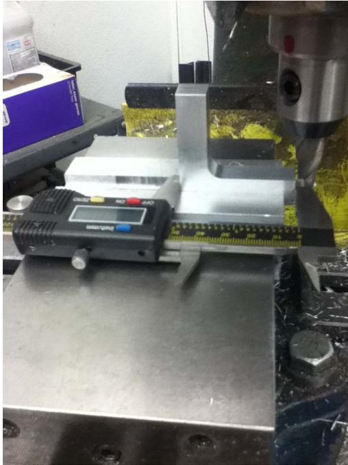
I could see that I had 0.247" to go. Two passes of 0.100" each got me down to about 0.05". Then I made a 0.030" pass before checking with the caliper again. The caliper showed I had 0.014" to go. I then took my first, calibrating, finish cut of 0.007". The caliper said I now had 0.007" to go. This told me that there was no need for a correction factor. I then dialed in my final 0.007" cut.
