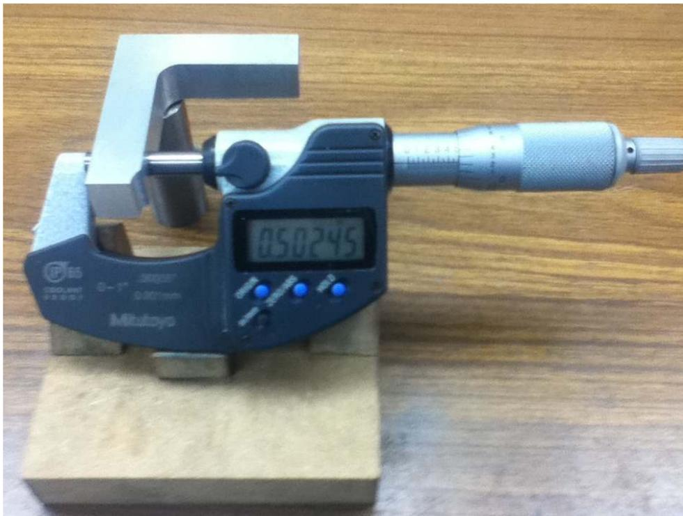
My first test is for the thickness of the longer leg. My micrometer is good to +/- 0.00005” and has been zeroed before use. I read 0.50245” so am 0.00245” too thick at this point. The test was repeated at two other spots along this leg and a maximum variation of 0.00015” was seen. I then repeated the test on the short leg and saw 0.050340” at the end with a maximum variation of 0.00015”. The absolute thickness error of 0.002” or 0.003” could easily be improved. The variation is good
