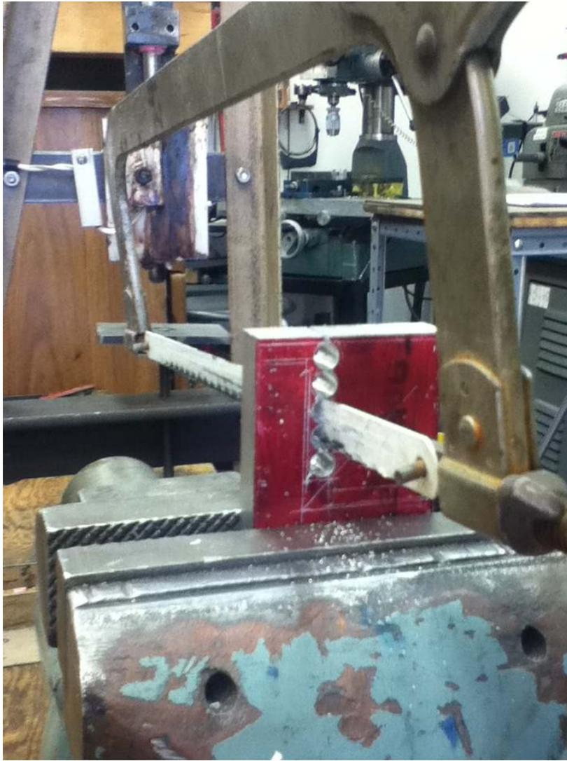
I'm using a 24 teeth per inch hacksaw blade to cut the web. It only takes one or two passes to clear each web.
