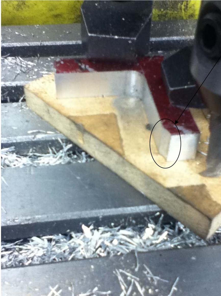
This is after the finish cut. You can clearly see that I almost got it right. The instant I fed in the cutter at what really was the right point (2"), I saw that I had taken a very big cut. I quickly backed out and then saw the wrong finish line so cut to it. This would have been fine if I had just realized which was the true finish line.
