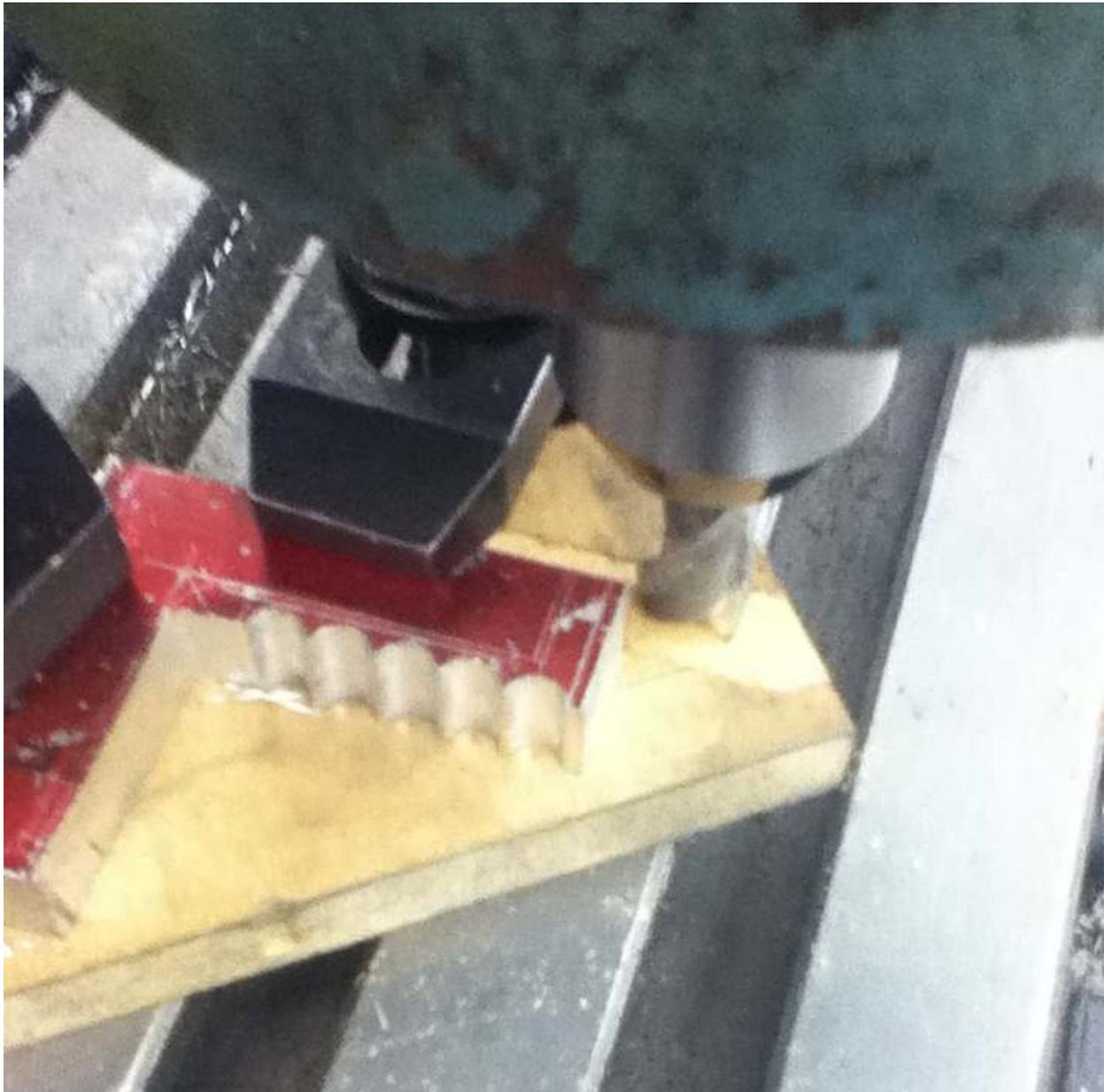
The clamps are then moved to the other side one at a time. I don't want the part to be completely unclamped and possibly shift.
