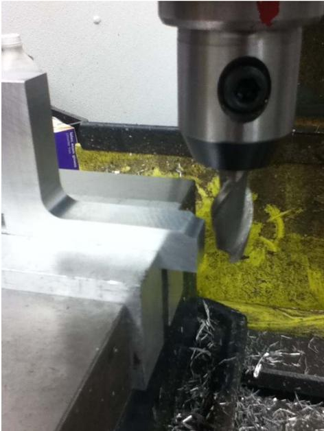
Although this is just a test part, it annoyed me to see that error in the longer leg. So I went back and fixed the mistake. First I clamped it into my vise and took a reference cut. I then set my DRO to zero.
