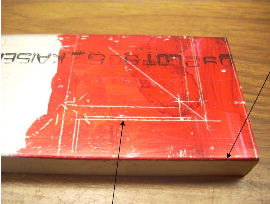
The bottom of the horizontal foot will ideally be the original edge of the plate. But if the plate is not perfectly aligned to my mill's axes, some cutting will be necessary to square up the part.
