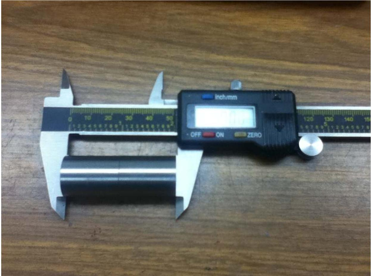
I also own a cheap Harbor Freight digital caliper. I zeroed the caliper on the two spacer blocks. In this way the readout will show me differences from 2.000". The caliper has its own error but experience has shown me that this error is small when movement is small. I am only expecting an answer to the nearest 0.001".
