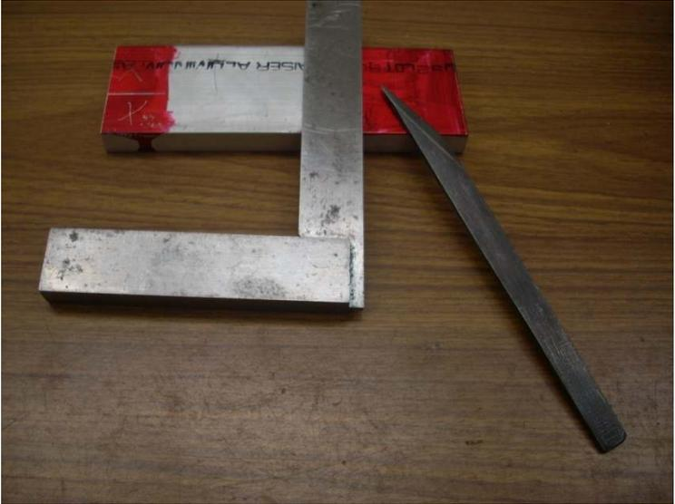
The bottom edge is reasonably straight and smooth so I will use my machinist square against it. Lines are scribed with a knife and very little pressure. The goal is to cut through the dye and not into the metal. I also used a 6" steel ruler that reads in decimal inches.
