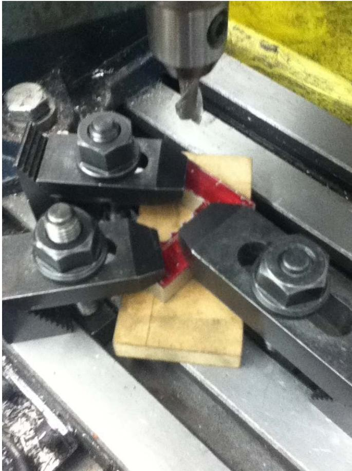
We are finally ready to run the mill. Since the inside corner is to have a 1/4" radius, I will use my 1/2" diameter end mill. It is mounted in an end mill holder which makes it convenient to install into my spindle.
