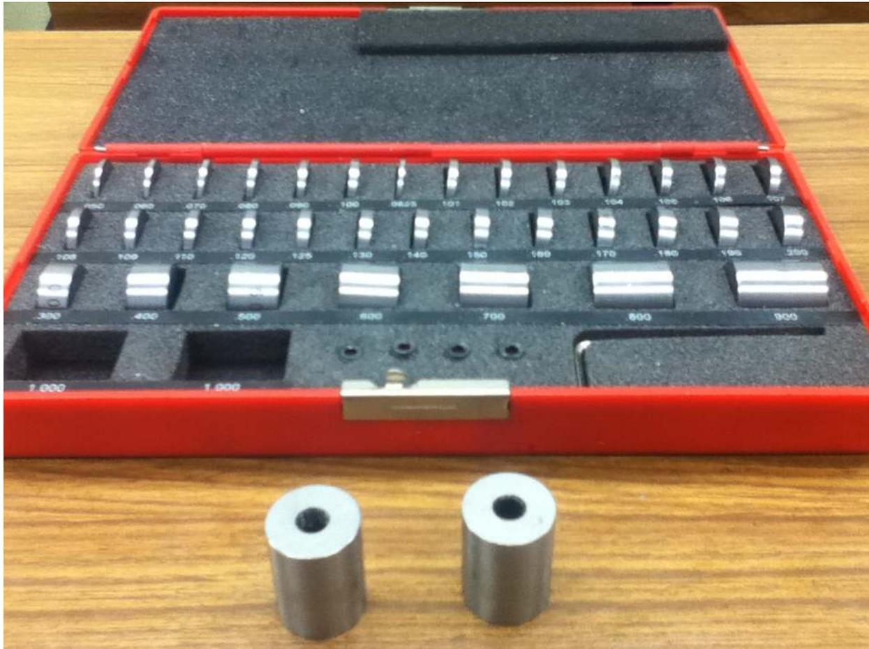
I own a set of what are called Spacer Blocks. These cylinders have a length accurate to  $\pm 0.0002$ ". I have removed two 1.000" blocks.
