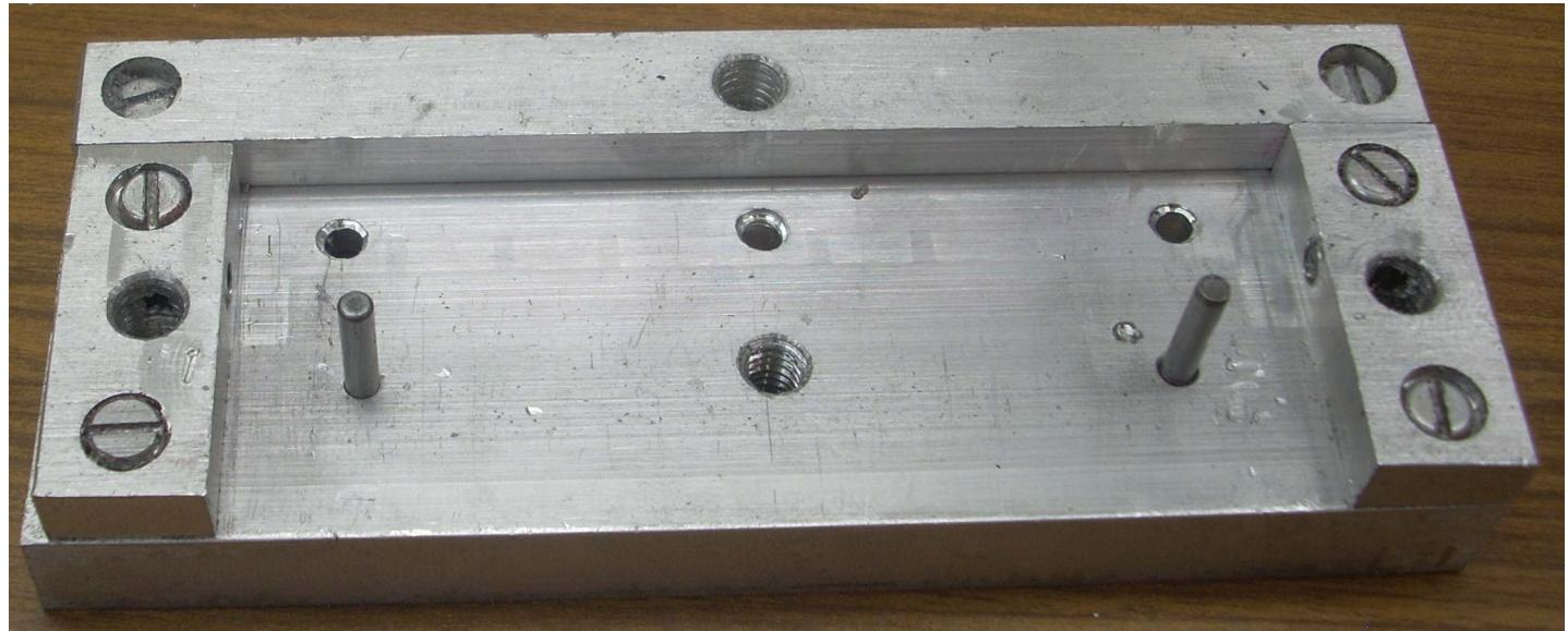
Two 1/8" dowel pins drop in first.
