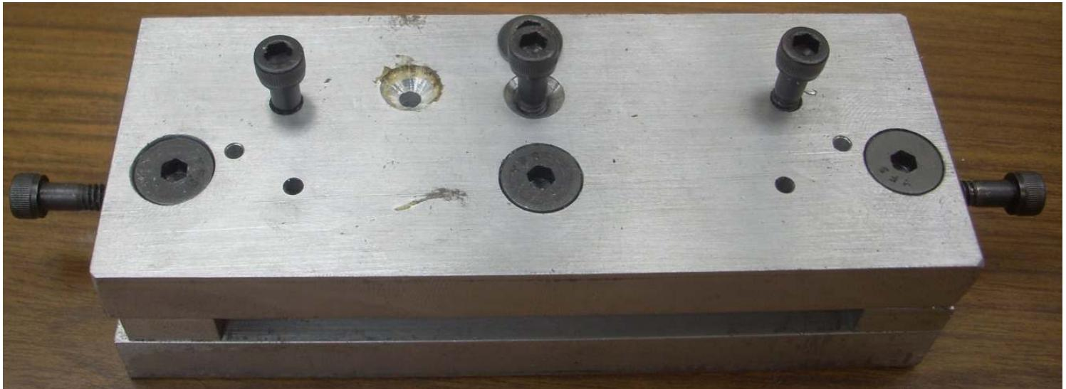
Note the hole between the left hold down bolt and the left top screw. This is where excess plastic will come out to tell me the void is full. This hole is called a riser. I have a second riser on the right side.
