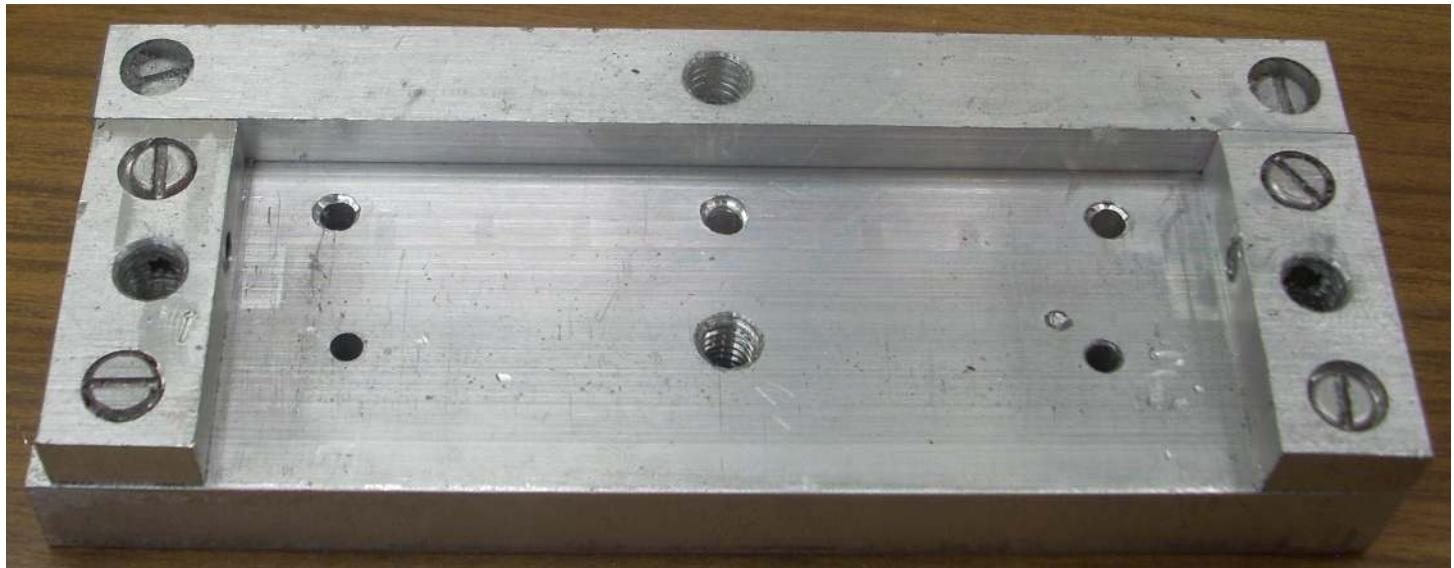
The drag (the bottom of the mold) was built up rather than machined out. After attaching these three pieces with 6-32 screws, I took a light cut across the top to insure they were at the same height. This is essential for a close fit of the cope (the top half of the mold). The location of the blocks was set by the insert which will be shown later.
