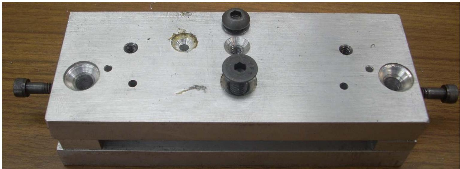
Next the two center locking  $\frac{1}{4}$ -20 screws go in. The back screw should have been a flat head rather than a button but it interfered with the filler nozzle on the molder. Later I had to move the filler hole (the sprue) so in the end, it didn't matter.
