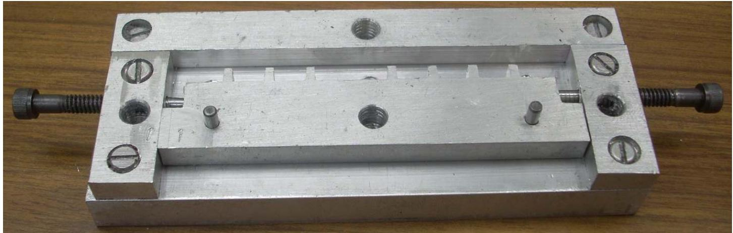
The side screws feed in until they contact the insert.
