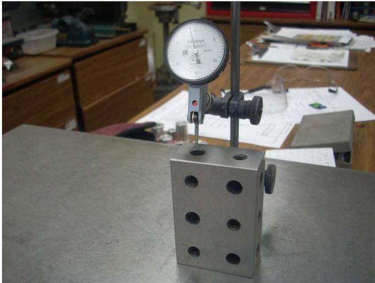
But this time the DTI reads - 0.001" which tells me the 2-3 faces are not as close to perpendicular to the X end as the non-X end. This is still rather good since this 0.001" error is the total error between two faces. So each face is off by 0.0005" over a distance of 3". That translates to an angle of 89.990°.
