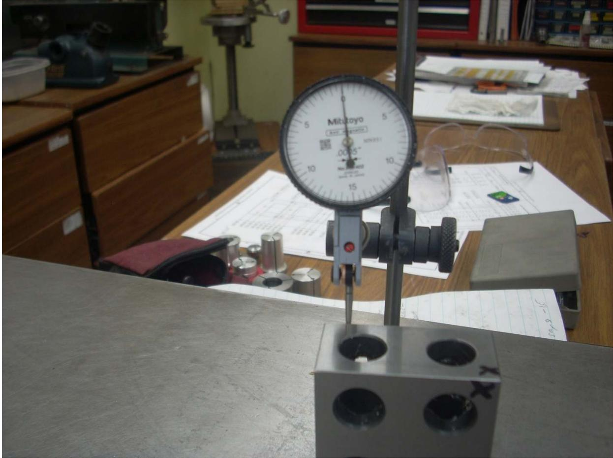
I again used the DTI support's fine adjust to move the finger into the block until it read zero. Note the two "X" marks on the front top corner. They will help us keep track of where we are on the block.
