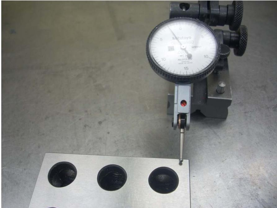
I start by setting the DTI dial to read about -0.002". This minimizes the spring tension on the finger when the DTI reads zero.
