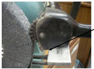
Removing the excess wheel material is easily done with a wheel dressing tool.
