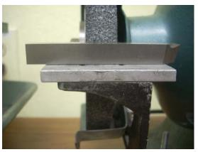
The dressing tool did a great job of getting the wheel close to true. I was able to get it a little better by following up by grinding the side of an old High Speed Steel tool blank.
