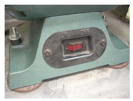
Mounting the grinder on rubber feet and sliding rubber grommets over the hold down bolts will reduce the amplitude of these table related resonances. But to minimize the vibration further, we must do more work.
